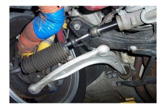
4. Undo the nut on the end of the steering rack shaft until it is completely disconnected. Do not change the position of the toe adjusting nut.
