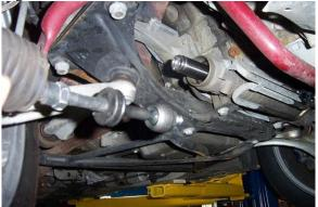
5. Take the appropriately colored rack stop, and evenly push it on the shaft until it is flush with the end of the shaft. The use of a block of wood and a hammer to evenly tap it on may be required.
