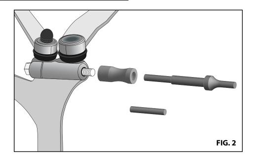
(This tool has been designed in pieces for ease of access, and it will require three steps to completely remove the pinch bolt)
