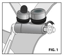
If necessary, rotate the steering wheel in order to access the pinch bolt with the Drift Tool mounted in an air chisel. Refer to **FIG. 1**, then loosen and remove the nut on the pinch bolt.
