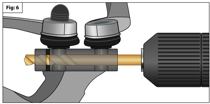
Use the 10mm Drill Bit to clean up any leftover burrs, corrosion, or debris from the bolt bore in the knuckle (**Fig: 6**). Pull the control arms out of the knuckle, remove any rust or corrosion from the knuckle and ball joints. Replace the pinch bolt and lock nut, coat the shank of the bolt with anti seize (not the threads), then torque them to specification.
