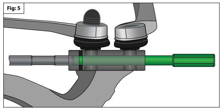
Loosen the M10x1.5x35mm Bolt and the 8mm Drill Bit Guide from the Clamp, and remove all three from the knuckle. Use the 10mm Punch and a hammer to remove the hollowed out pinch bolt (Fig: 5).
