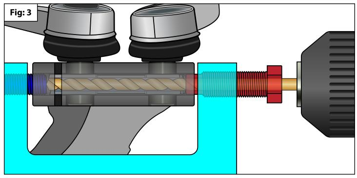
Place the 6mm Drill Bit into a power drill, then slide the bit through the 6mm Drill Bit Guide and drill a hole all the way through the broken pinch bolt (Fig: 3).
