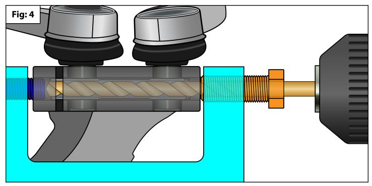
Remove the **6mm Drill Bit Guide** from the **Clamp** and replace it with the **8mm Drill Bit Guide**. Slide the 8mm Drill Bit through the **8mm Drill Bit Guide** and drill a hole all the way through the broken pinch bolt (**Fig: 4**).
