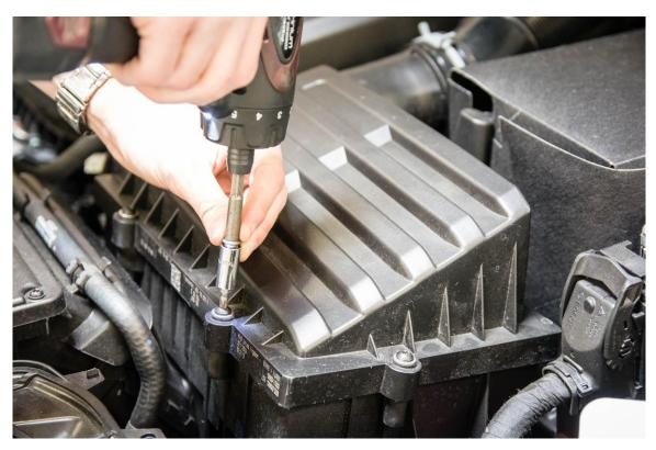
**Step 3** – Remove the breather hose from the front left side of the factory airbox.
