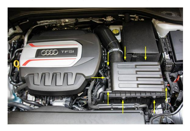
**Step 2** – Using the T25 Torx bit, loosen and remove all 8 screws securing the upper airbox to the lower airbox. Set 6 of the screws aside for reinstallation of the 034Motorsport MQB P34 Intake System.
