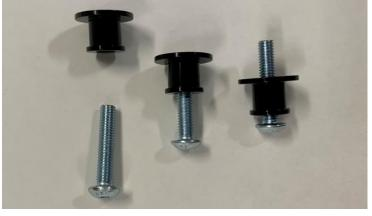
**Step C** Secure spacers to X34 airbox with M5 locking nuts and 8mm deep socket.
