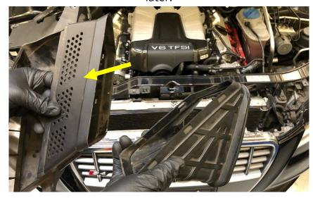
**Step 5**Remove the Rear Engine cover and set aside gently.
