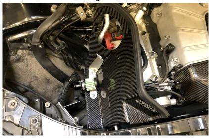
**Step 13**Install the secondary air hose to the adapter.
