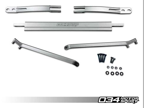
034Motorsport's Billet Aluminum Front Strut Brace for the B8 Audi Q5 & SQ5 is designed to limit lateral deflection from the strut towers and improve handling performance without sacrificing ride quality or introducing any additional noise, vibration, or harshness into the cabin.
