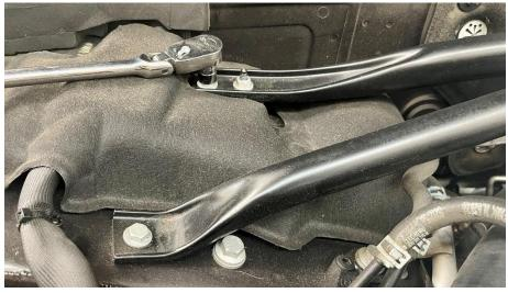
**Step 3** Using a 10mm socket, remove the nuts from the firewall brackets.
