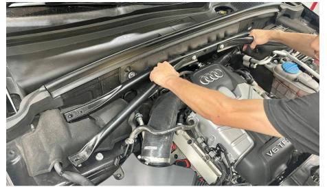
**Step 5** Carefully place the assembled 034 strut brace into location.
