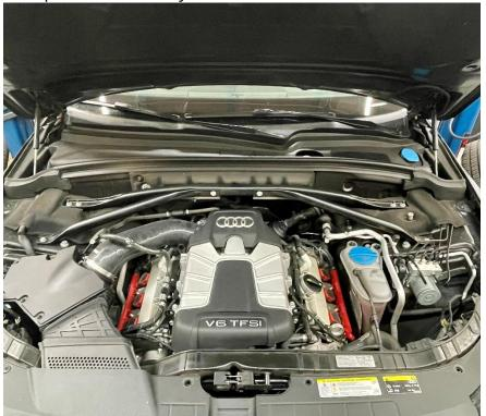
Step 2 Using a 13mm deep socket, remove the 4 nuts and 2 bolts securing the factory strut bar.
