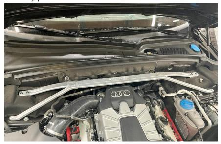
Use the provided M8 washers and nuts to secure the primary supports to the chassis.
