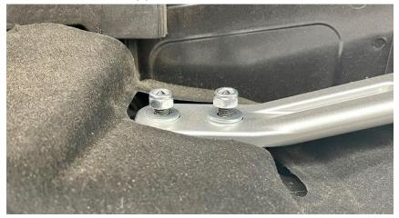
**Step 7** Use a 6mm Allen on the provided M8 bolts to secure the secondary supports to the chassis.
