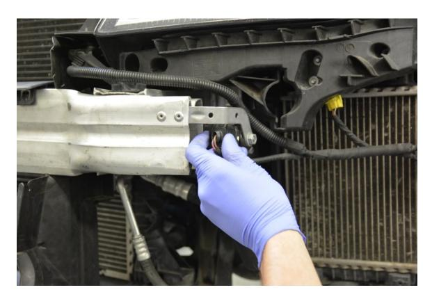
**Step 9** – Disconnect right side horn, and wire retaining clip.
