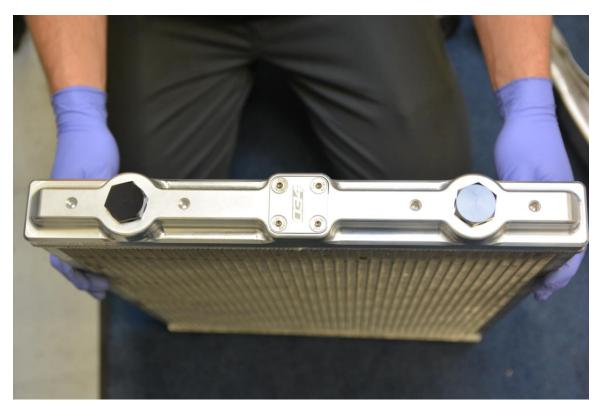
**Step 18 –** Install mounting brackets using M8x14 button head cap screws and M8 lock washer. Blue Loctite can also be added to screws. **Note:** bracket to bumper bar mounting flange points outward from heat exchanger.
