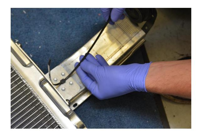
**Step 27 -** Assemble air block-off plates.
