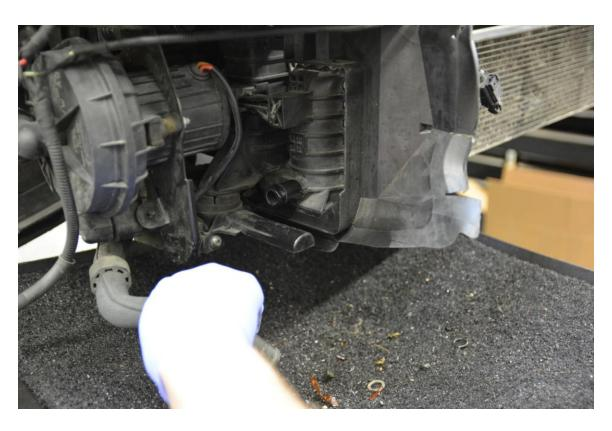
**Step 4** – Placing a suitable catch pan underneath, remove upper heat exchanger hose using pliers, or spring clamp pliers.
