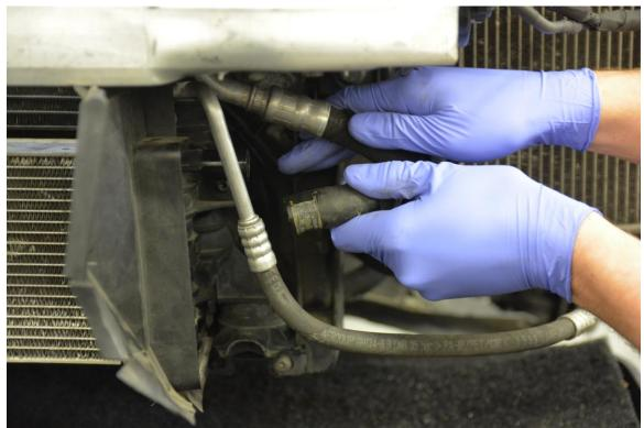
**Step 5** –Using the T30 Torx bit, unbolt the factory heat exchanger. Screw is on left hand end only.
