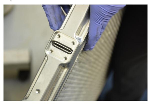
**Step 15a (B8.5 only)** – Insert diverter plate in driver side (RHD cars) end tank to create dual-pass unit.
