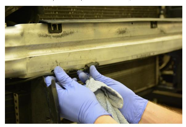
**Step 11** – Using 13mm socket, remove (4) M8 bolts securing bumper bar. **Note:** you may have to pry between the bumper bar and frame rails to loosen enough to slide out.
