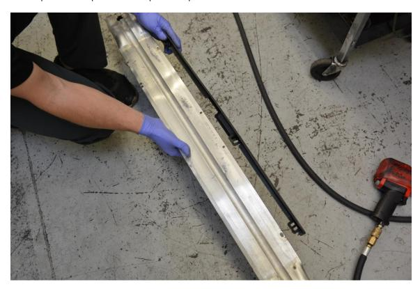
**Step14a -** Install 25x3 o-ring in groove in 034 heat exchanger end tanks.
