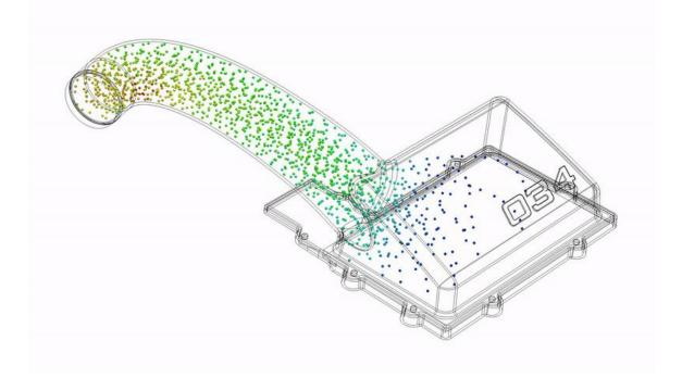
034Motorsport's mechanical engineers scanned the factory engine bay and modeled a one-piece unit to replace the factory intake tube and upper airbox. By eliminating the multiple couplers, transitions, and jagged features in the factory upper airbox and intake tube, 034Motorsport's engineering team was able to drastically reduce turbulence in the intake tract, and virtually eliminate pressure drop in the intake system before the turbo inlet.
