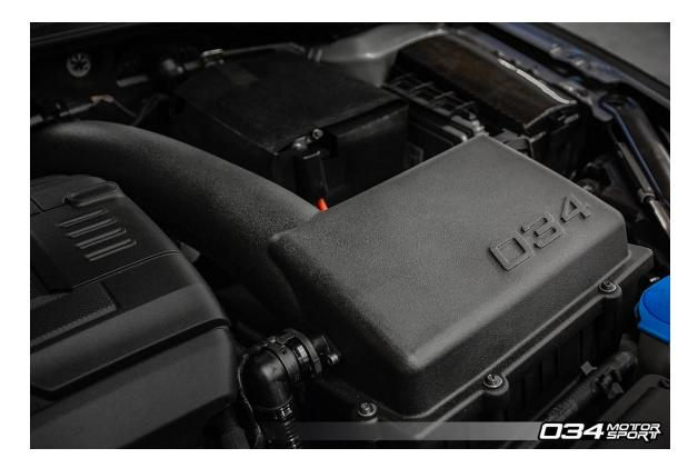
To ensure that the P34 Air Intake System draws in cool, dense air, 034Motorsport engineers opted for an enclosed design to prevent hot air from the engine bay entering the intake tract. By bolting to the factory lower airbox, this approach allows the enclosed high-flow panel filter to breathe fresh, cold air from the factory inlet duct before the radiator.
