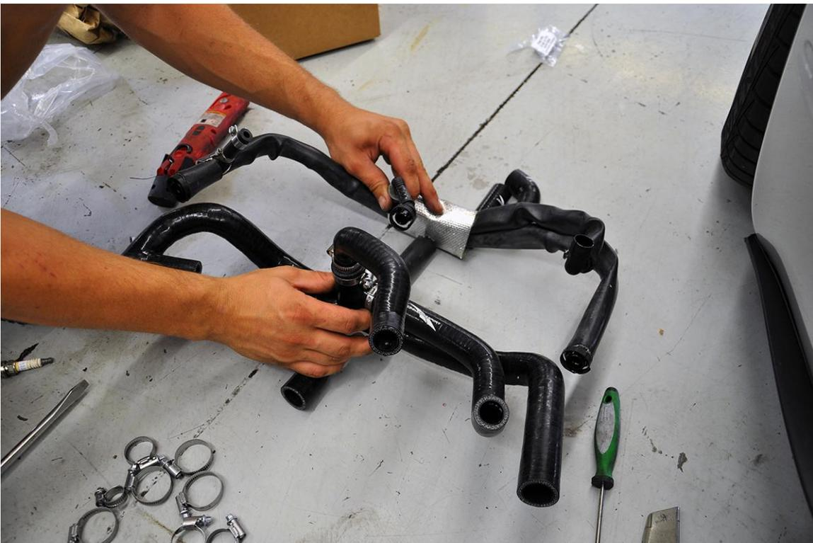
**Step 11** – Slip the Silicone Spider Hose into place. Install the block breather hose first, clamping it securely once the hose is properly aligned.
