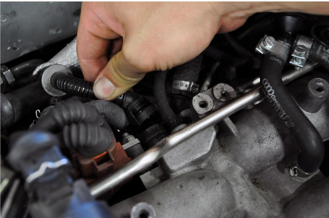
**Step 7** – Remove the PRV from your spider hose assembly. You can use the box cutter to make this easier. At this point, you can reuse the factory (clip) connection to the y-pipe, or use our supplied Early PRV Hose or Late PRV Hose.
