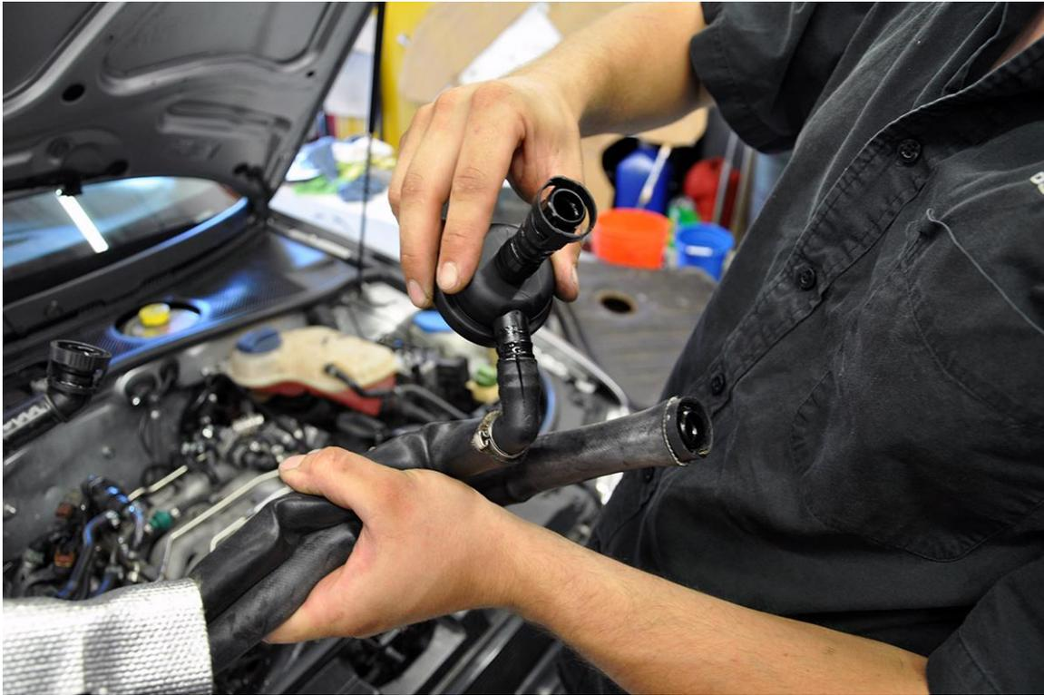
**Step 8** – Replicate your spider hose using the hoses supplied in our kit, which are pictured and labeled below.
