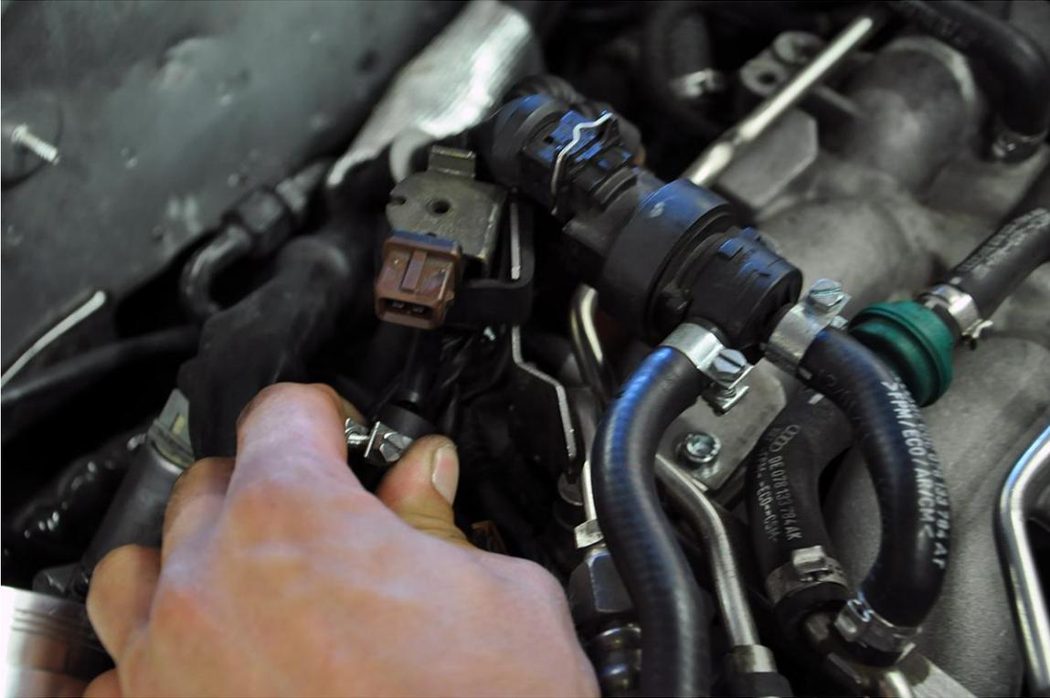
**Step 6** – Disconnect the breather hoses running from the factory spider hose to the intake manifold and block. By now you should be an expert at removing these things without breaking them. Congratulations! You can now remove the spider hose from the engine bay.
