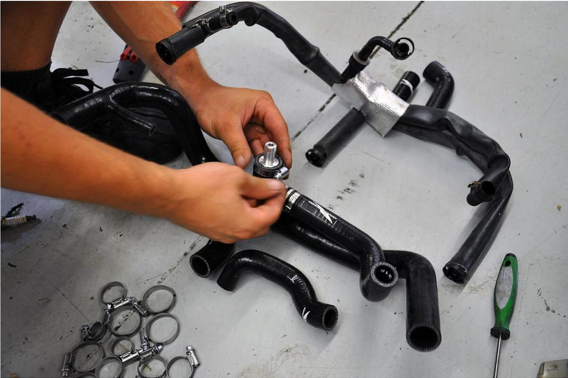
**Step 10** – The picture below is of an assembled late breather hose system, which mimics the factory spider hoses. If you end up with a silicone hose that looks like the plastic piece you removed, you're on the right track! Clamp the check valve to intake manifold hose lightly, as you may need to rotate it during installation.
