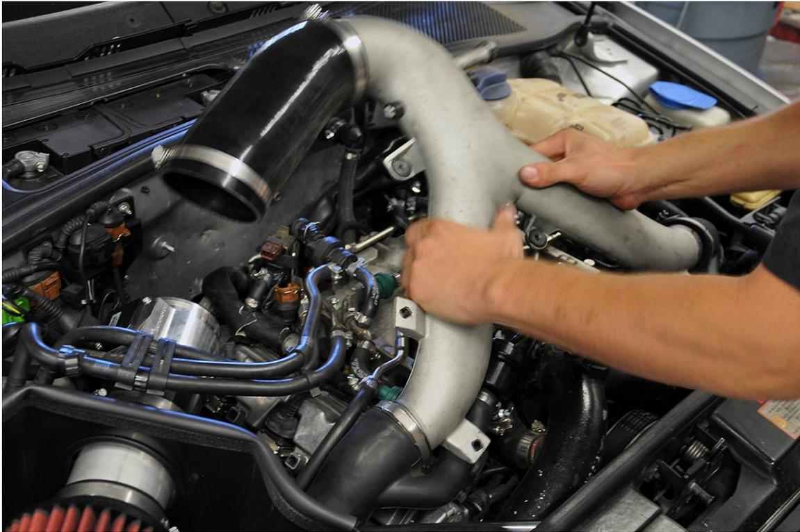
**Step 4** – Remove the valve cover breather hoses from both valve covers.
