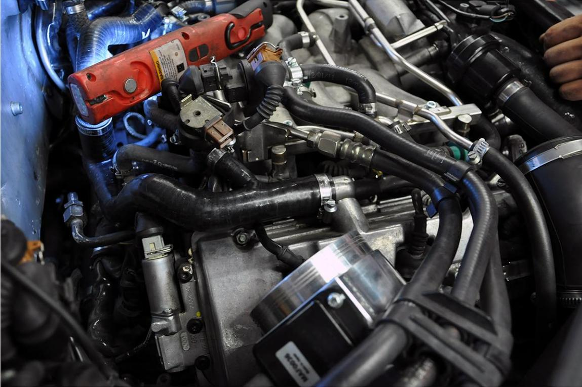
**Step 14** – Connect the hose from the billet check valve to the intake manifold. This may require you to rotate the hose on the clamp slightly. Tighten both clamps.
