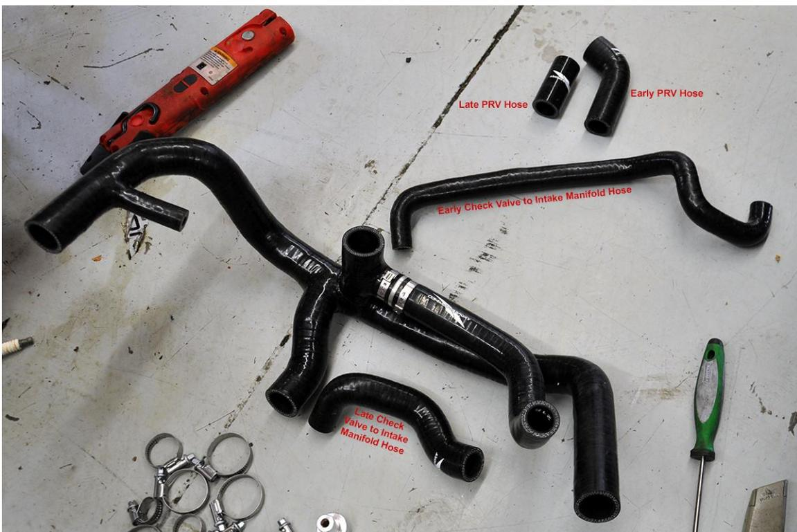
**Step 9** – Install the supplied 034Motorsport Billet Check Valve into the Main Breather Hose Assembly as pictured below. Clamp securely using supplied hose clamps.
