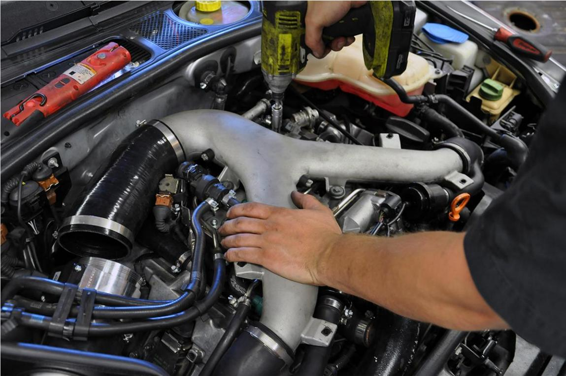
**Step 16** – Install the PRV into the spider hose assembly. Using either the factory connector or the one of the supplied silicone hoses, attach the PRV to the y-pipe.
