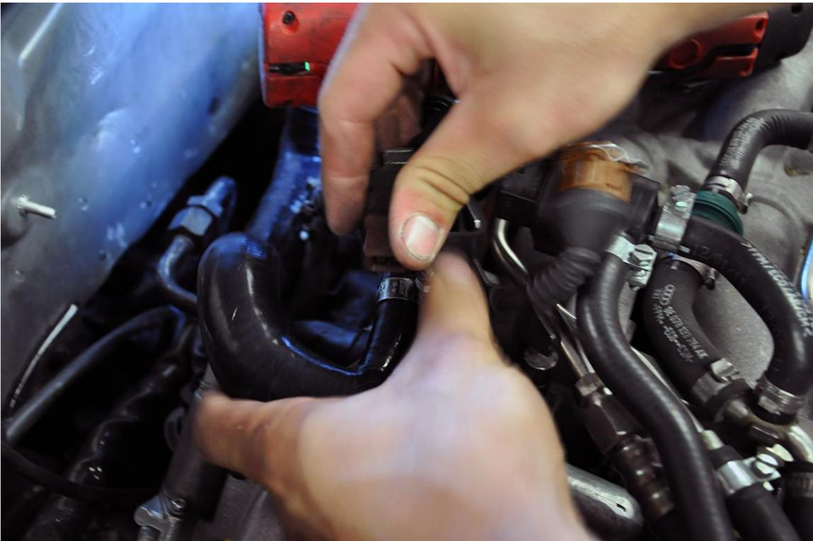
**Step 13** – Connect the two valve cover breather hoses to the valve covers, and clamp them securely. Plug in the N75 valve's 2-pin connector.
