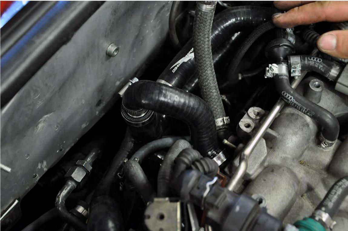
**Step 15** – Reinstall the y-pipe, making sure to use the three 10mm bolts and clamp all hose connections securely.
