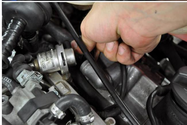
**Step 5** – Unplug the electrical connector to the N75 valve. Remove the vacuum hose below the connector that goes to the N75 valve.
