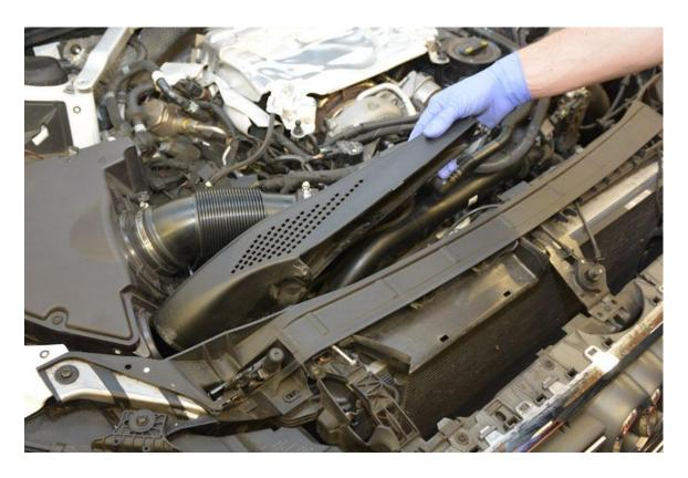
**Step 7** – Using a 7mm socket, loosen the hose clamp attaching the air filter hose from the turbo inlet pipe.
