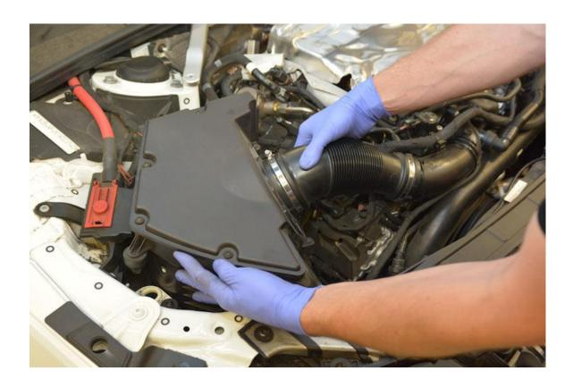
**Step 9** – Transfer the 3 rubber mounts from the stock airbox, to the 034Motorsport X34 Carbon Fiber Cold Air Intake.
