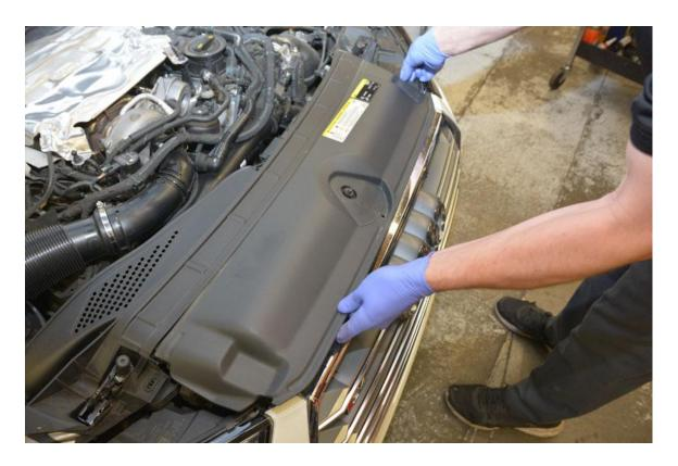
**Step 5** –Using the T25 Torx bit, unscrew the two screws holding the factory air duct to the radiator support.
