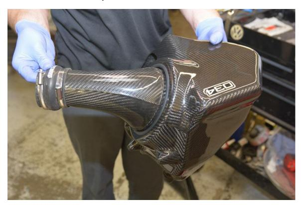
**Step 11** – Install assembly, connecting inlet tube to turbo inlet, and pushing down on airbox to insert rubber mounts into receptor holes.
