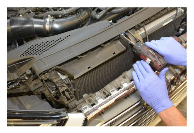
**Step 6** – Remove air duct.
