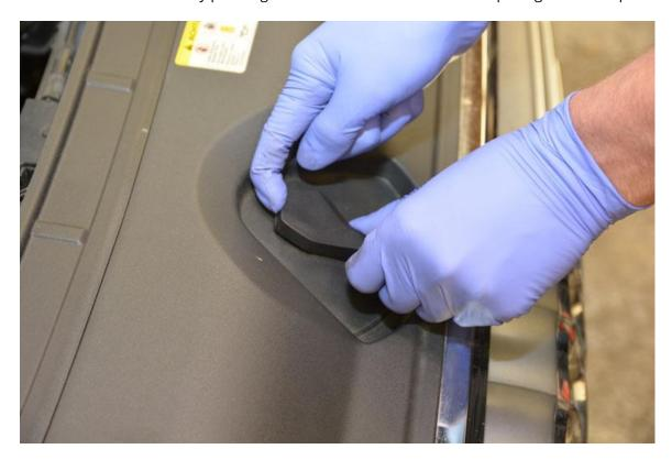
**Step 4** – Remove cover by gently prying up on front edge to release clips, and slide forward and out.
