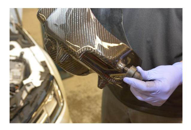
**Step 10** – Install intake tube/filter assembly into airbox.
