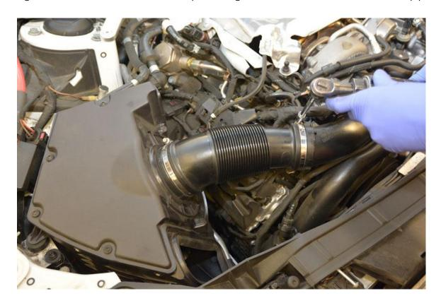
**Step 8** – Remove the airbox from the car by simply lifting up and out.
