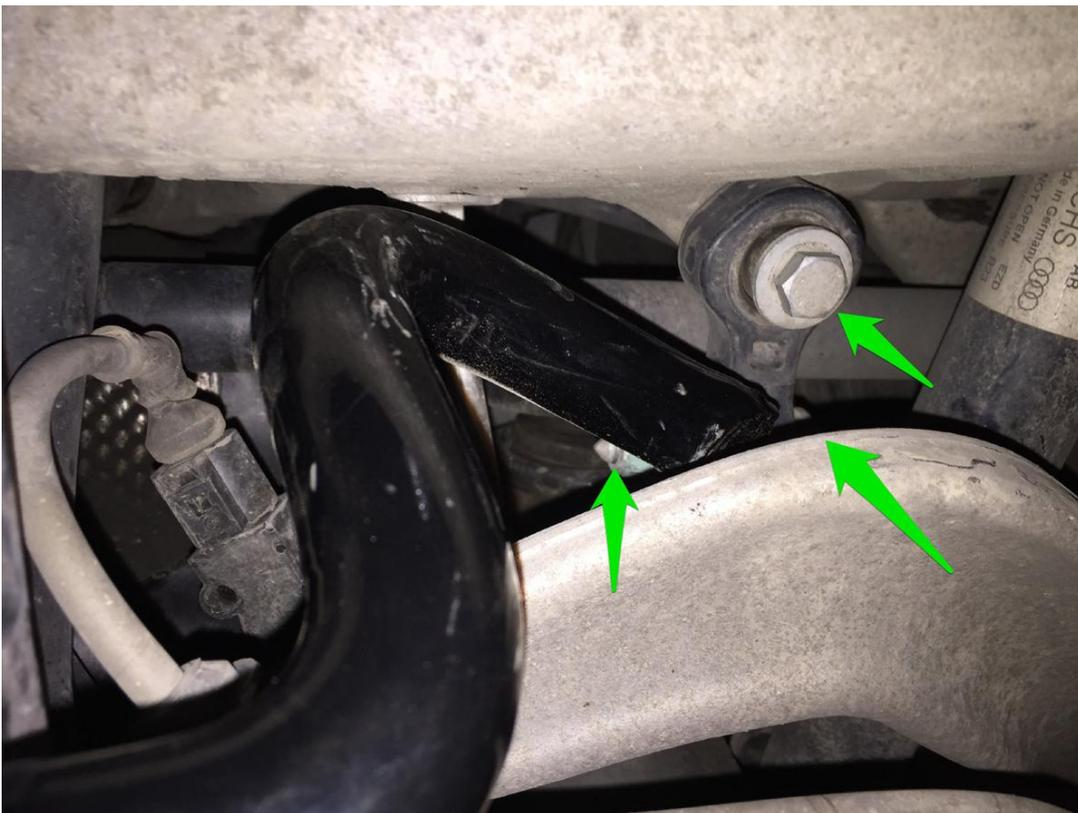
**Step 9** – Torque the sway bar end link hardware to 40 Nm + 90 Degrees. **Please Note:** We recommend replacing the factory end link bolts as they are torque-to-yield bolts.
