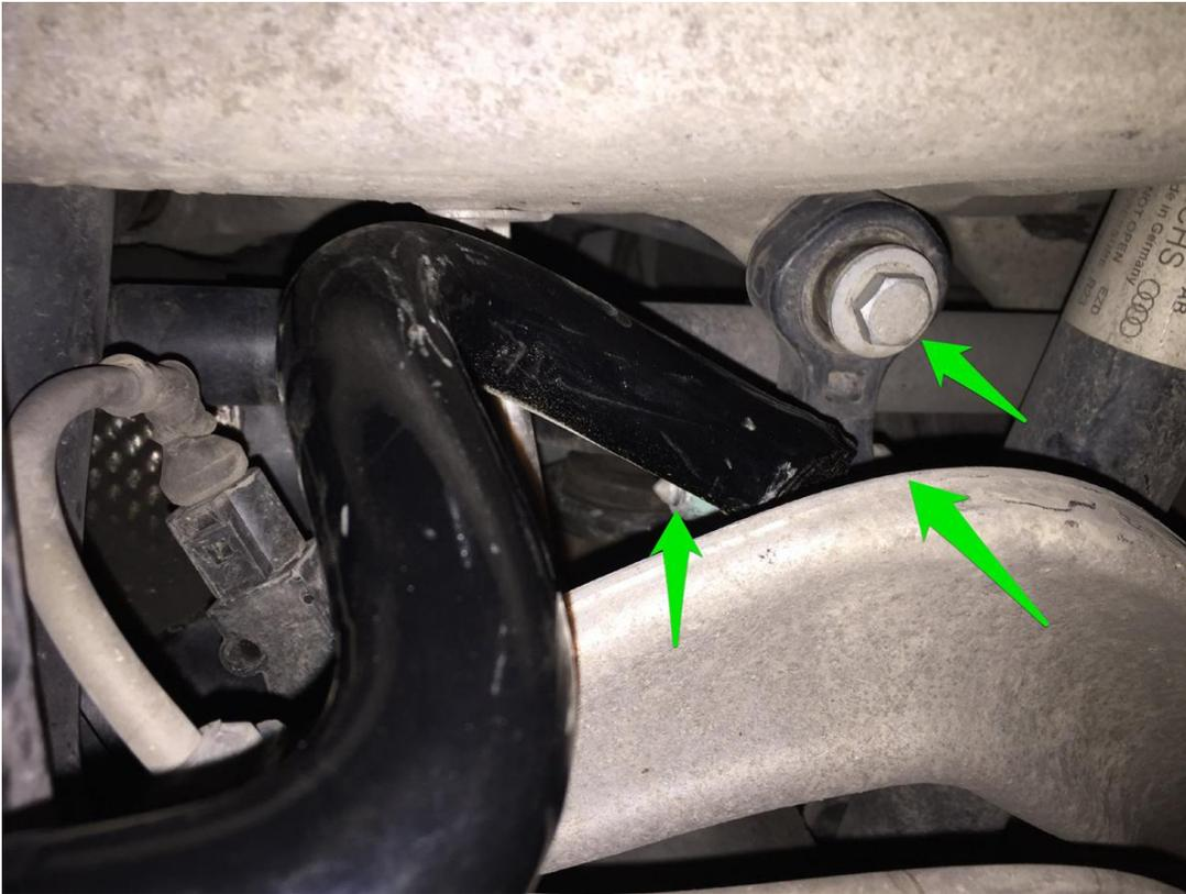
**Step 10** – Tighten the sway bar mount bracket bolts to 28 Nm.
