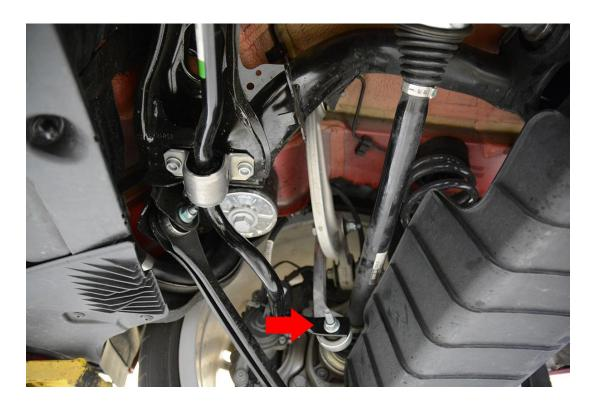
**Step 2** – Remove the triple square bolts securing the factory sway bar mounting brackets to the rear subframe.
