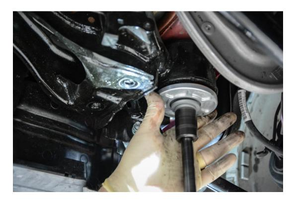
Step 10 - Torque to 130 NM + 180 Degree Turn.
