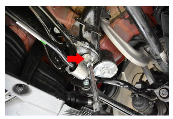
**Step 3** – With the sway bar mounting brackets and end links removed, snake out the rear sway bar from underneath the vehicle.
