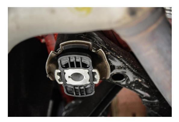
**Step 14 –** The rear bushing of the rear subframe should resemble the photo below.
