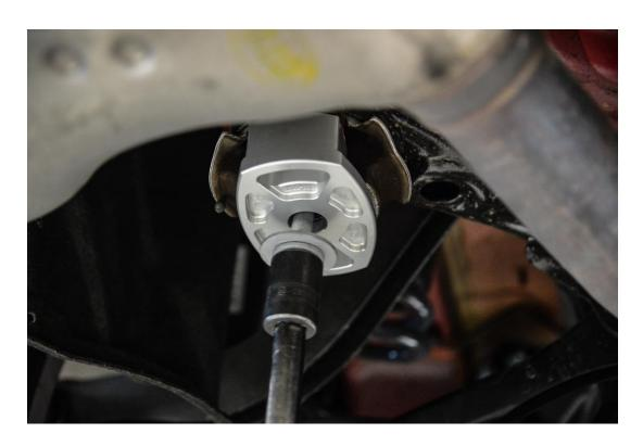
**Step 17 –** Repeat steps 4 through 17 to install the remaining 034Motorsport Billet Aluminum Rear Subframe Inserts for the other side of the rear subframe.
