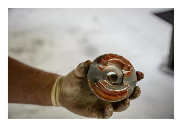
**Step 9** – Insert the Front 034Motorsport Billet Aluminum Rear Subframe Bushing Insert into the factory rubber bushing, and secure using the factory subframe bolt and a 21mm socket.
