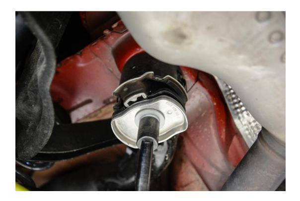
**Step 12** – With a pry bar, remove the factory metal retainer from the rubber bushing.
