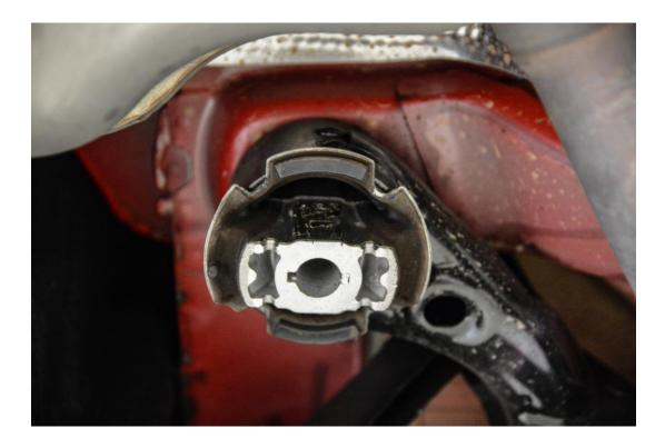
**Step 15 –** Apply a coat of grease to the Rear 034Motorsport Billet Aluminum Rear Subframe Insert. (PN: 601-0045)
