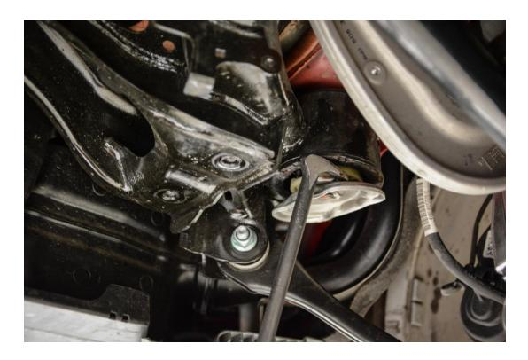
**Step 6** – Finally, remove the factory plastic retainer from the rubber bushing.
