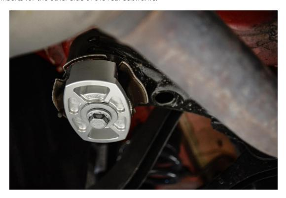
**Step 18 –** Once all four 034Motorsport Billet Aluminum Rear Subframe Inserts are installed and torqued to spec, reinstall the rear sway bar, beginning with the mounting brackets. **Note:** Hardware may differ from factory rear sway bar for aftermarket bars.
