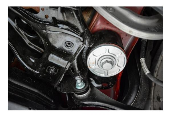
**Step 11** – Using an 18mm socket, loosen and remove the factory bolt securing the rear bushing of the rear subframe to the chassis.
