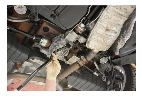
**Step 4** – Using a breaker bar and 21mm socket, loosen and remove the bolt securing the front subframe bushing.
