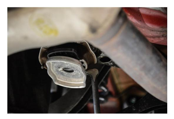
**Step 13 –** Remove the black plastic collar from the rubber bushing.
