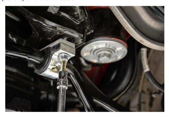
**Step 17 –** Reattach rear sway bar to rear sway bar end links. Torque end link hardware to **40Nm + 180 Degree Turn**. Torque rear sway bar mounting bracket bolts to **28 Nm**.
