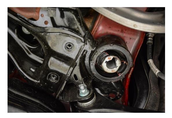
**Step 8** – Apply a thorough coat of grease to the Front 034Motorsport Billet Aluminum Rear Subframe Mount Insert. (PN: 601-0044)
