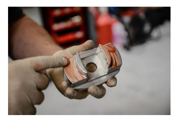
**Step 16** – Insert the Rear 034Motorsport Billet Aluminum Rear Subframe Bushing Insert into the factory rubber bushing, and secure using the factory subframe bolt and an 18mm socket. Torque to **90NM + 180 Degree Turn.**
