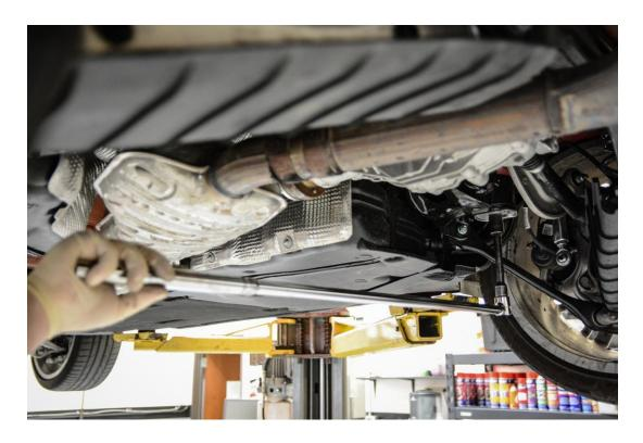
**Step 5** – Once the bolt is removed, use a pry bar to remove the factory metal collar from the rubber bushing.
