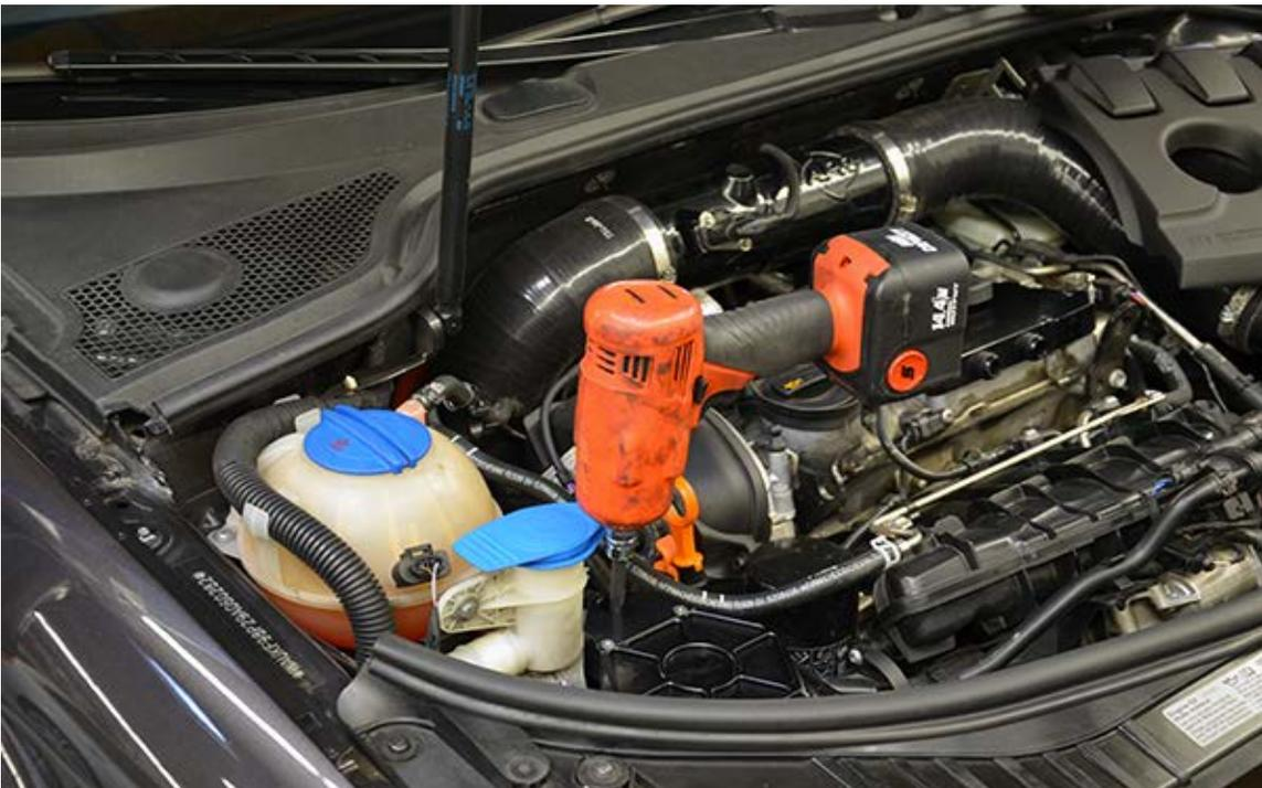
**Step 12** – Route the -10 AN Breather Hoses as pictured below, and secure to the Valve Cover Breather Adapter and Catch Can. Install the hose separator over the hoses and secure using the Allen bolt as pictured.
