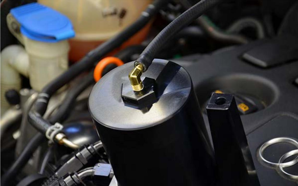
**Step 2** – Route the line for the oil drain away from any belts and pulleys, and secure it using the provided zip-ties. It needs to run from the catch can to the oil drain plug on your oil pan.
