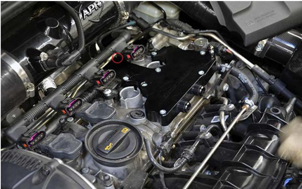
**Step 9** – Plug the coil harness back into all four coils, and secure the loom using the factory T30 Torx screw. Reinstall the coilpacks.
