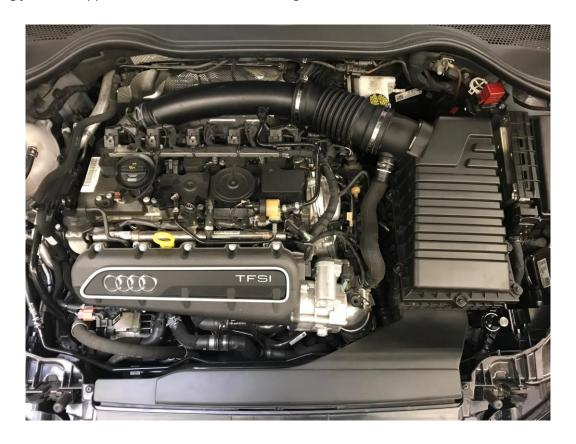
**Step 3** – Using a pair of pliers, loosen the spring clamps on the bypass hose and disconnect hose from OE intake.
