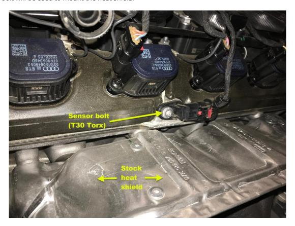
**Step 9 -** Using a 4mm Allen wrench and the supplied M6 button head cap screws, assemble heat shield.
