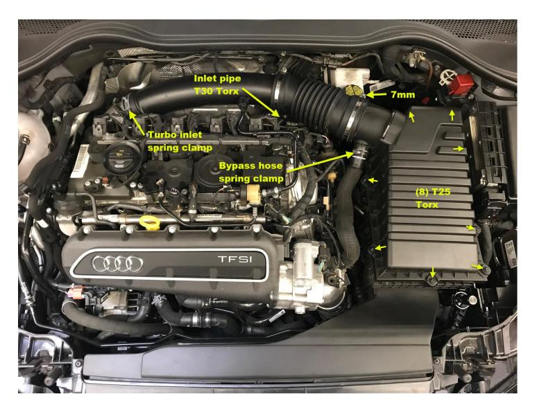
**Step 4** – Using the same set of pliers, loosen the spring clamp at the turbo inlet and slide the clamp up the inlet pipe and off the coupler (see image above).
