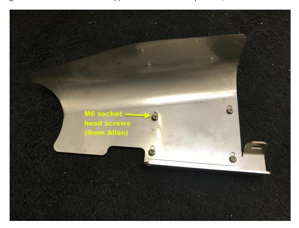
**Step10 -** Install the heat shield by attaching to the stock inlet tube mounting bracket (Step 6), and the head sensor (Step 12). Shield location can be adjusted by loosening the M6 button head cap screws. Make sure wiring along the firewall does not contact the edge of shield.
