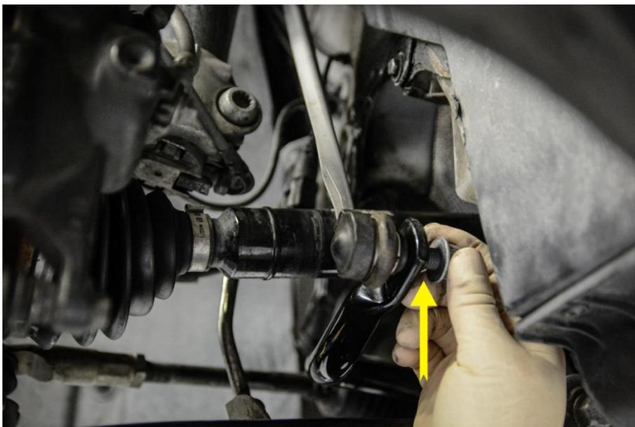
**Hint:** The outer hole is the "Soft" setting, and the inner hole is the "Stiff" setting.
