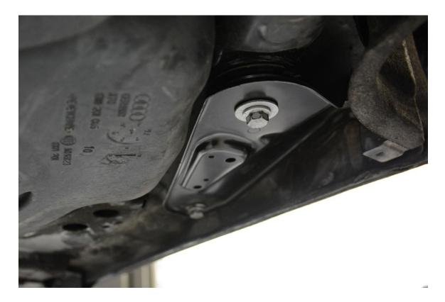
**Step 15** – Using a 16mm Socket, remove the two bolts securing the subframe mount bracket to the chassis.
