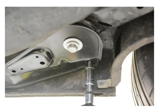
**Step 23** – Slide the rear subframe cover back into place, and secure using the three 10mm nuts and two T20 Torx screws.
