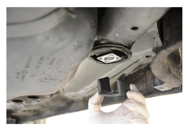
**Step 19** – Apply silicone grease to the insert as pictured below.
