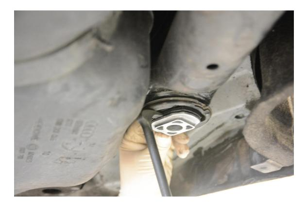
**Step 18** – Remove the factory plastic isolator and set aside.
