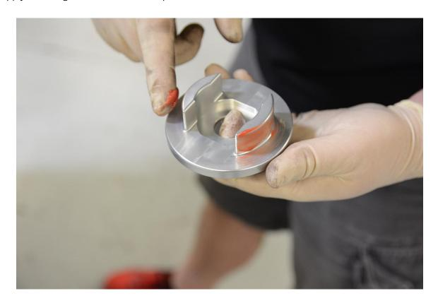
**Step 6** – Align the 034Motorsport Rear Subframe Insert (601-0034) with the voids in the factory subframe bushing.
