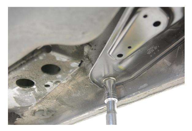
**Step 16** – Using an 18mm Socket, remove the bolt securing the front of the rear subframe to the chassis, and remove the steel subframe mount bracket.
