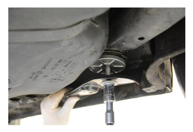
**Step 22** – Align the subframe mount bracket and reinstall the two 16mm bolts. Torque to 16mm bolts 55 Nm. Torque new subframe bolt to 115 Nm + 90° Turn. **If you opt to reuse the stock subframe mount bolt, torque to 120 Nm with Blue Loctite.**
