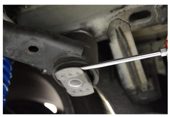
**Step 4** –Remove the factory washer and set aside.
