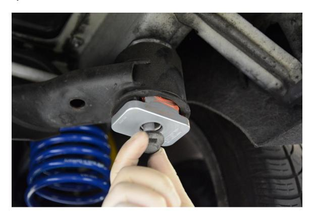
**Step 7** – Torque new subframe bolt to 60 Nm + 90° Turn. **If you opt to reuse the stock bolts, torque them to 90 Nm with Blue Loctite.**
