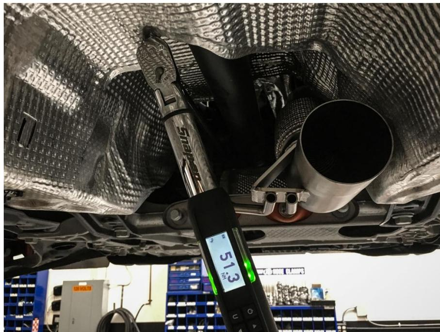
**Please Note:** We recommend replacing these bolts after removing. The part number for factory bolts is N90846102.
