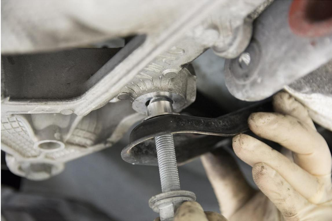
**Step 14** -Slip in spacing washers between the Steel Subframe Bracket and Body at the two rear holes, as shown below.
