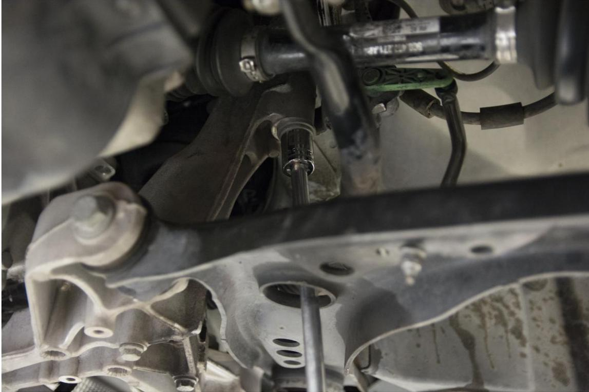
**Step 6** -Gather the Subframe Locking Collars. The 601-0026 are rear uppers, the 601- 0029 is front uppers, and the 601- 0027 are the four lowers. They must be installed in the correct locations!
