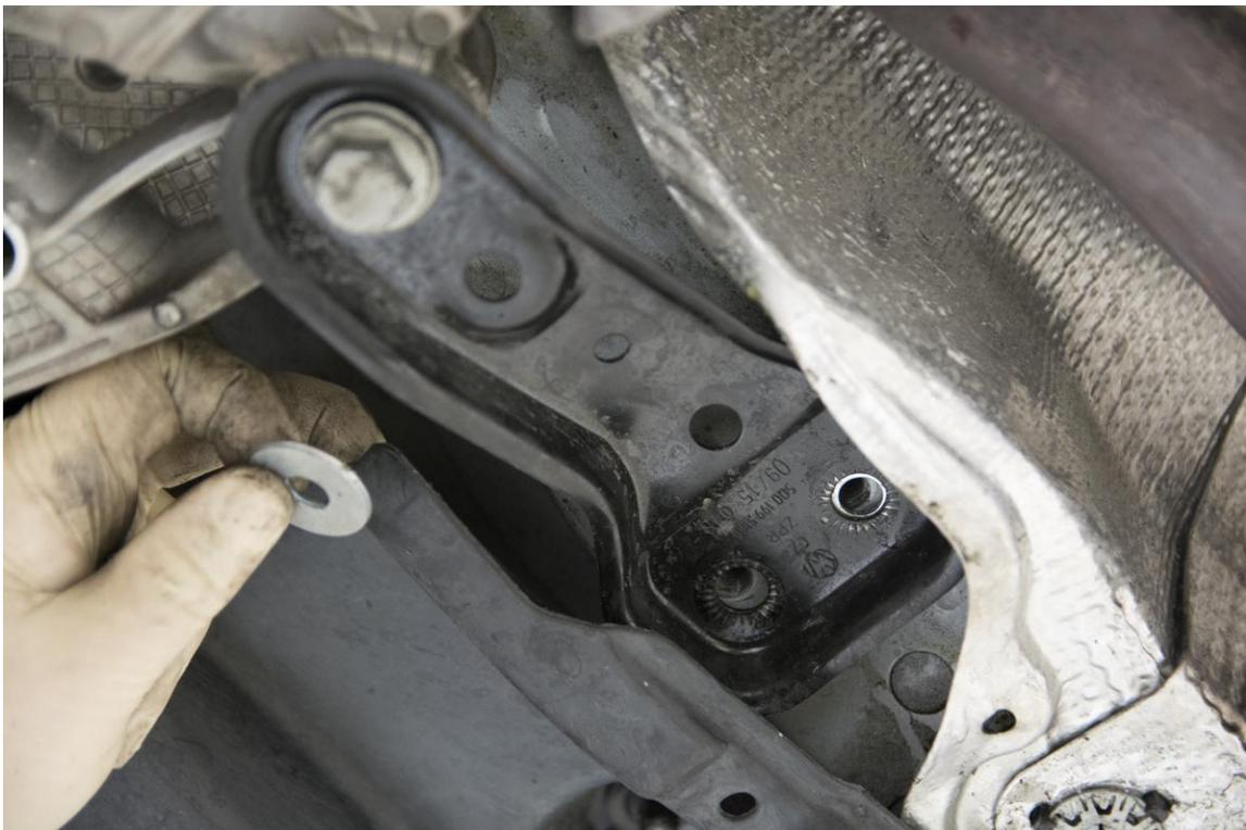
**Step 15** -With the spacing washers installed, reinstall the factory bolts removed in Step 3. Torque to 45 Nm with blue loctite.
