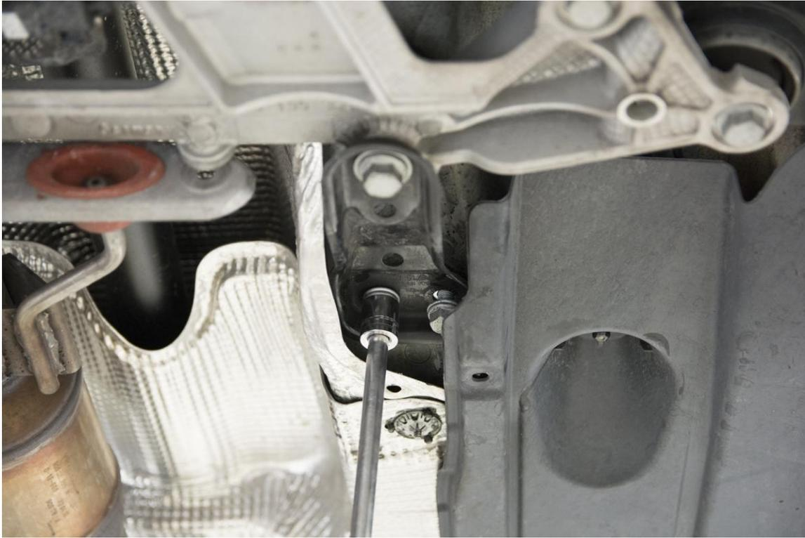
**Step 16** - Reinstall the two bolts securing the dogbone mount to the transmission. Torque to 50 Nm with blue loctite.
