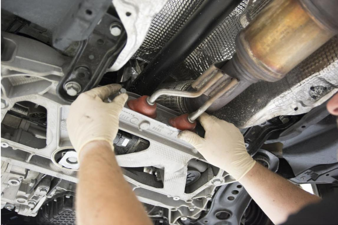
**Step 18** – Verify that the subframe is properly aligned and all Locking Collars are fully seated. Torque the new Factory Subframe Bolts to 70 Nm + 180 Degrees.
