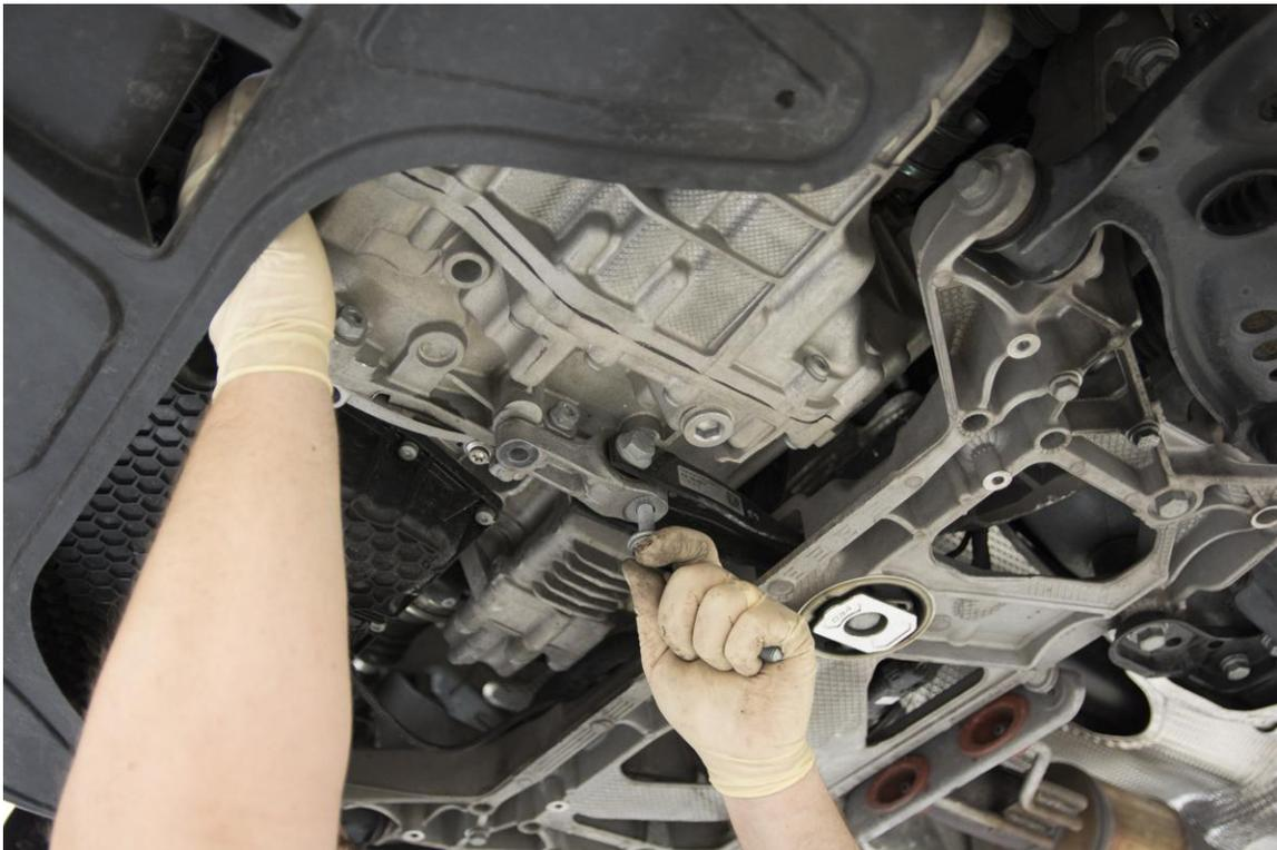
**Step 17** – Reinstall the bolts securing the factory exhaust hanger to the subframe. Torque to 20 Nm.
