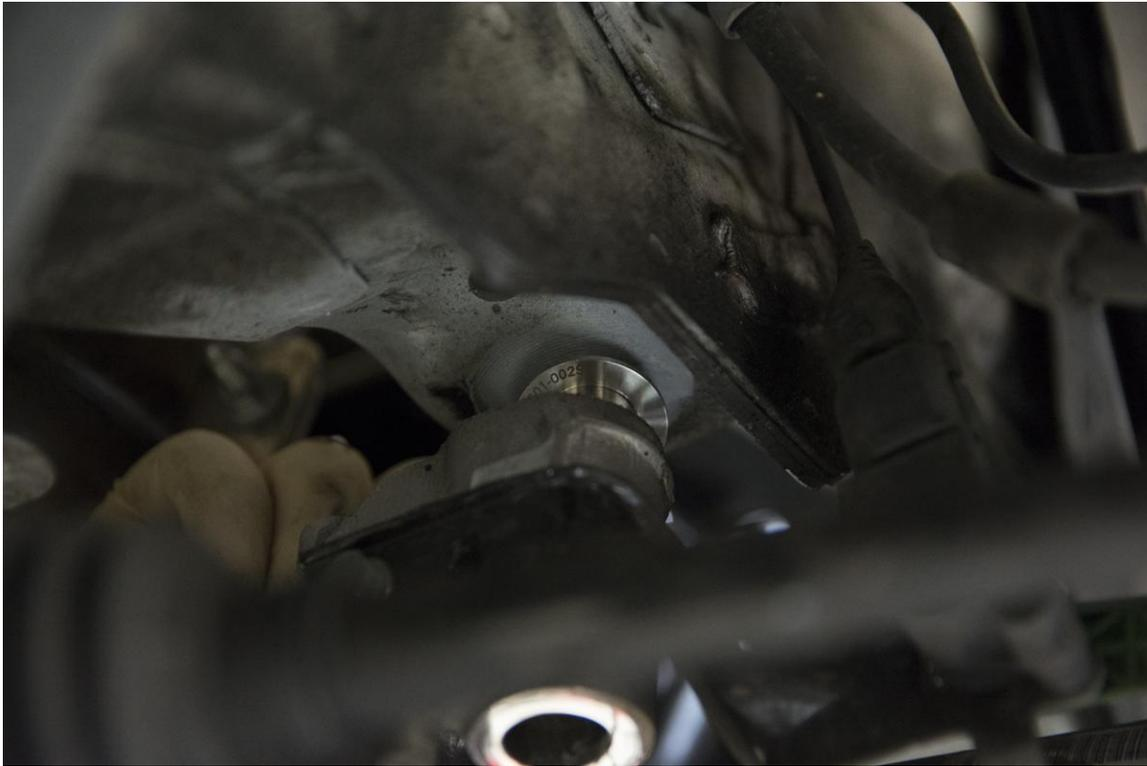
**Step 10** – Preinstall two of the 601-0027 Locking Collars onto the supplied new Factory Subframe Bolts, as pictured below.
