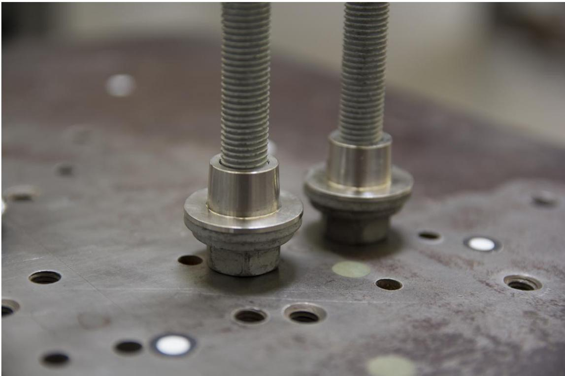
**Step 11** – Raise the subframe, and patiently install the new Factory Subframe Bolts with 601-0027 Locking Collars as pictured below. Take care to ensure that all four subframe holes are aligned, with the locking collars properly seated at the body. Do not fully torque these bolts yet!
