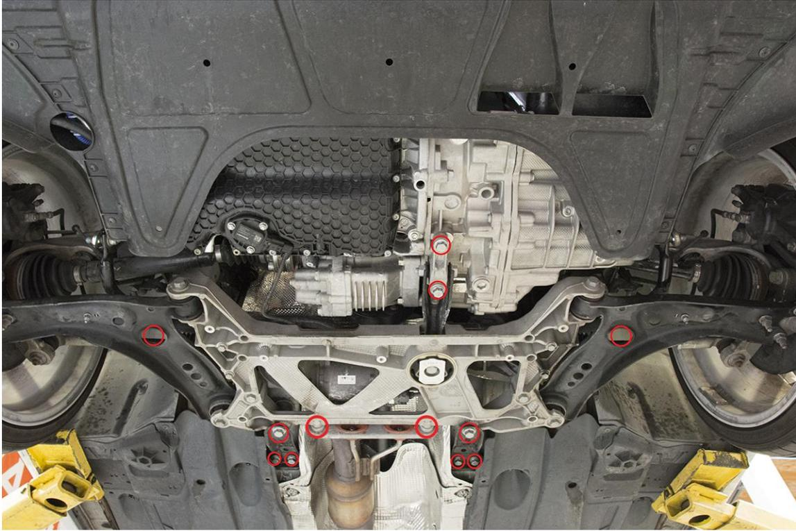
**Step 2** - Using a 16mm Socket, remove the two bolts securing the dogbone mount to the transmission.
