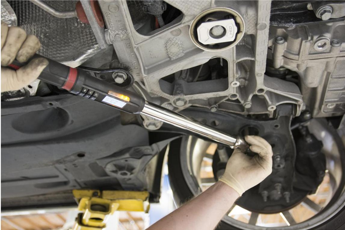
**Step 20** – Verify that all bolts have been torqued to spec and that the subframe is properly aligned with all Locking Collars fully seated. **Perform an alignment!**
