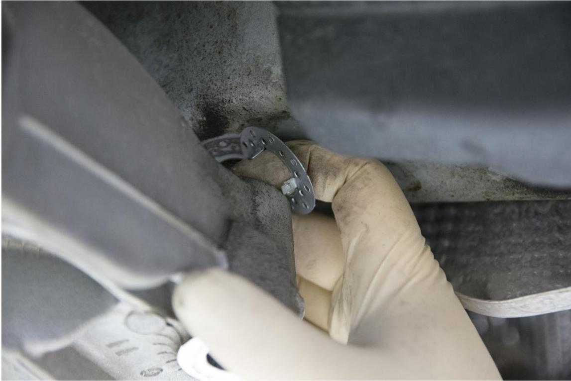
**Step 8** – Install the two 601-0026 Locking Collars into the tops of the rear subframe holes, as pictured below.
