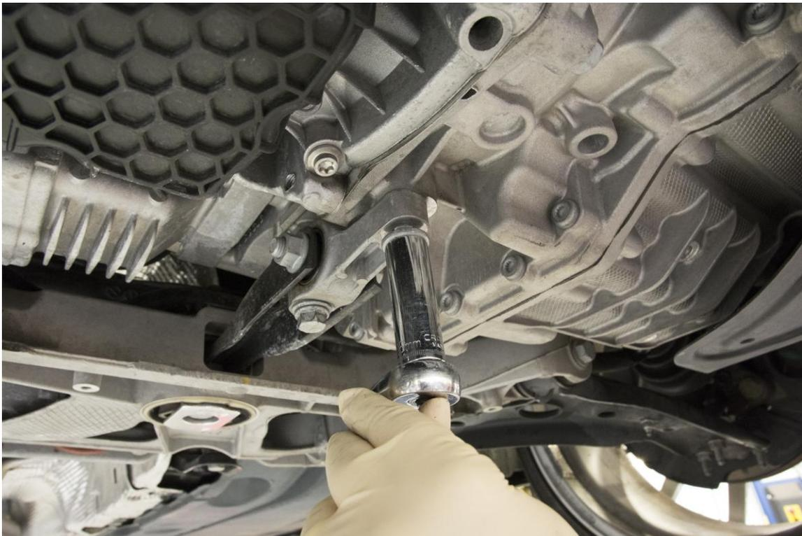
**Step 3** – Using a 16mm Socket & 18mm Socket, remove the bolts securing the steel subframe brackets to the subframe and body. Set the brackets and smaller bolts aside.
