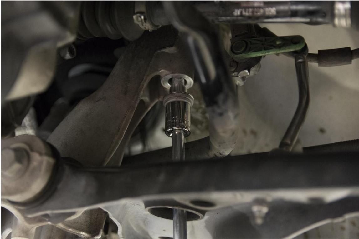
**Step 12** – Preinstall two of the 601-0027 Locking Collars onto the Steel Subframe Brackets and insert the supplied Factory Subframe Bolts, as pictured below.
