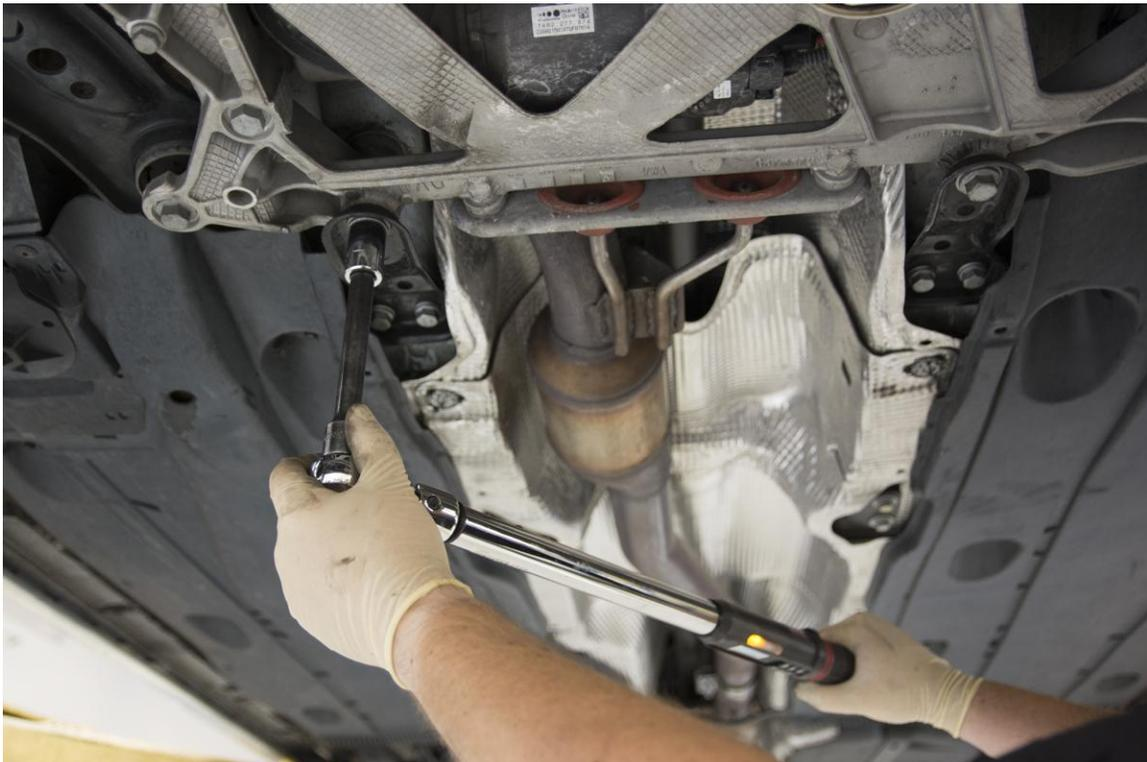
**Step 19** – Verify that the subframe is properly aligned and all Locking Collars are fully seated. Torque the new Factory Subframe Bolts to 70 Nm + 180 Degrees.
