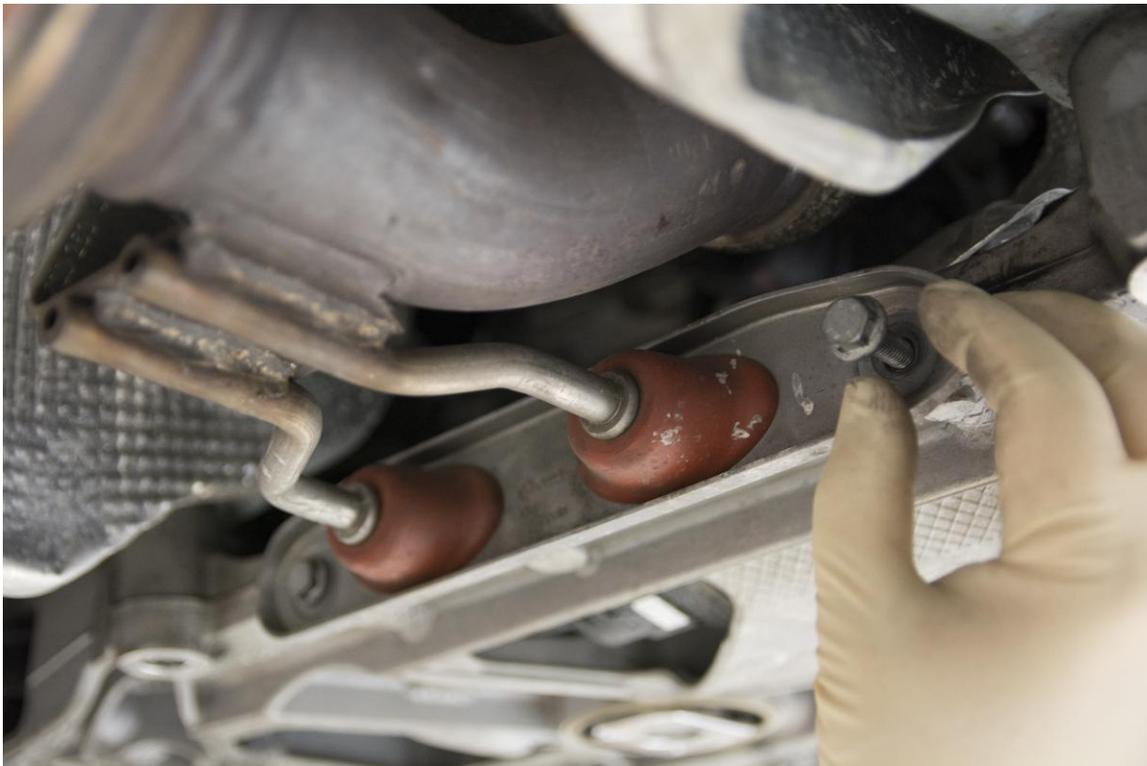
**Step 5** -Using an 18mm Socket and extension, remove the front subframe bolts.
