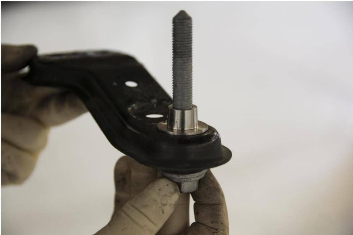
**Step 13** -Reinstall the Steel Subframe Brackets and loosely thread in the Factory Subframe Bolts, ensuring that the Locking Collars seat properly.
