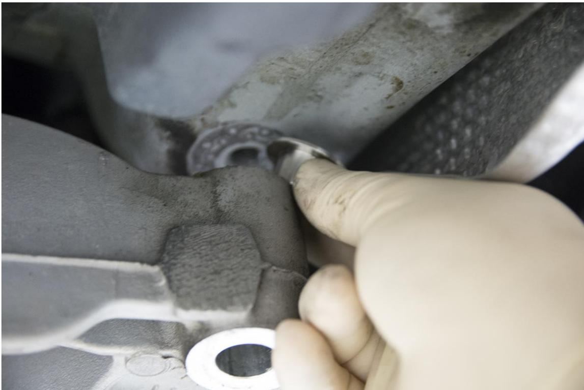
**Step 9** – Install the two 601-0029 Locking Collars into the tops of the front subframe holes, as pictured below.
