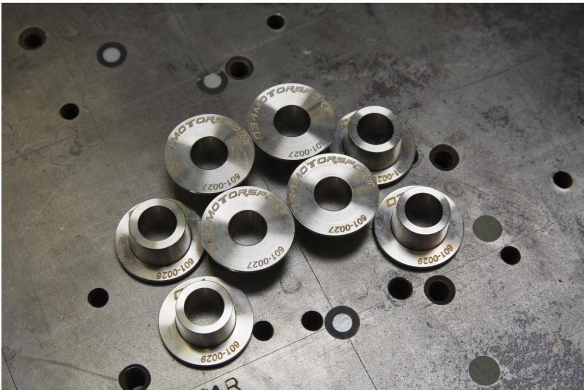
**Step 7** – Lower the subframe to allow for space to install the Locking Collars. Remove the steel shims from the top of the rear subframe holes, as pictured below.
