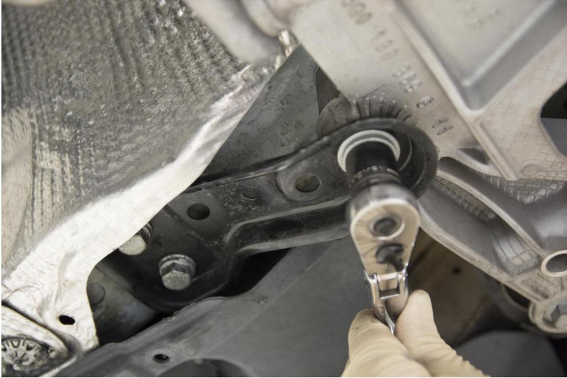
**Step 4** –Using a 13mm socket, remove the bolts securing the exhaust hanger to the subframe.
