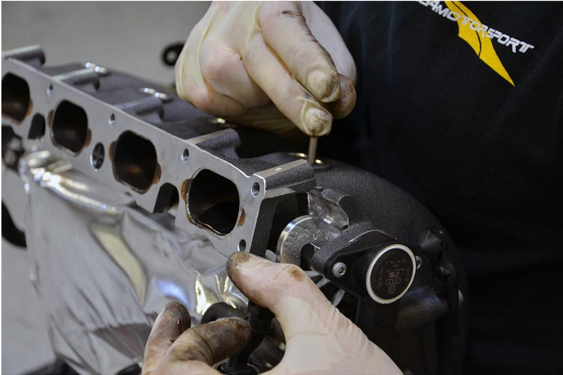
**Step 20** – Apply Loctite to the intake manifold plugs you removed in [Step 1](#), and gently tap them in using the shorter (small) end of the supplied Intake Manifold Plug Installation Tool. **Do not use the longer end for this!** The stop on the short side is designed install at the exact depth necessary for a proper seal. **Pressing the plugs too far in can result in them entering the intake tract!**
