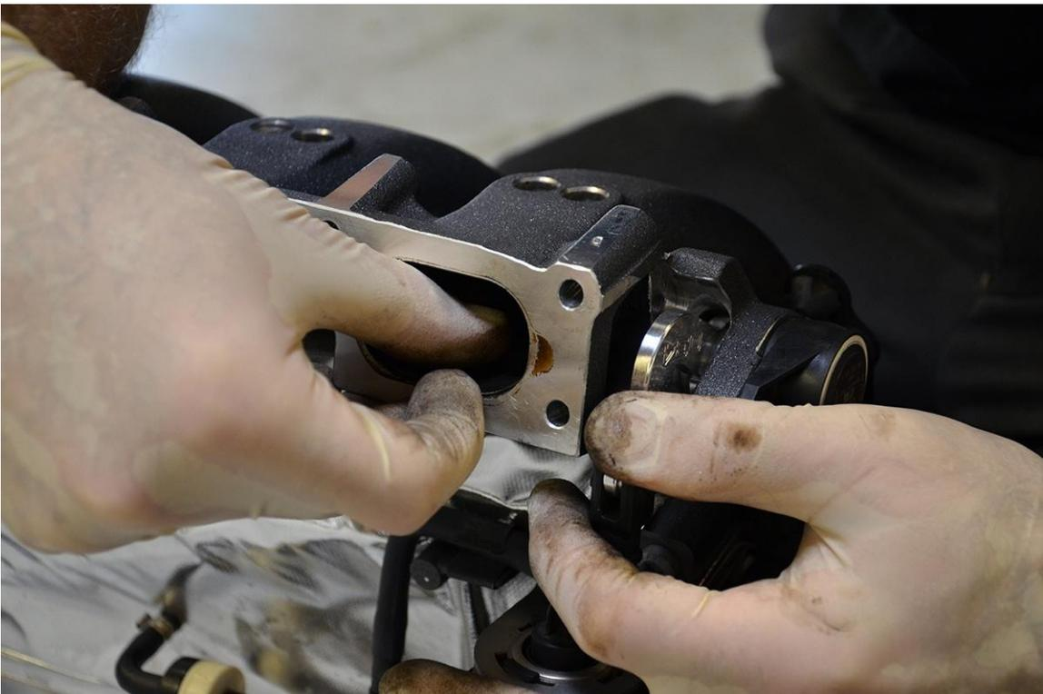
**Step 19** – Apply Loctite to the threads of the T20 Torx screws you removed from the intake manifold flaps/rods in [Step 3](#), and use them to secure the flaps to the rod.
