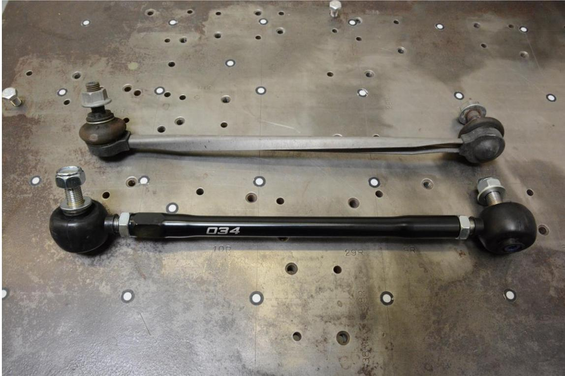
**Step 8** – Insert machined steel adapters into heim joints.
