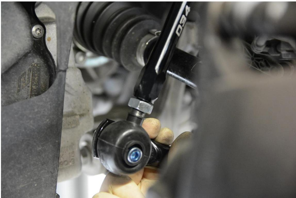
**Step 15** – Repeat installation on the other side, and verify that all hardware is properly torqued.
