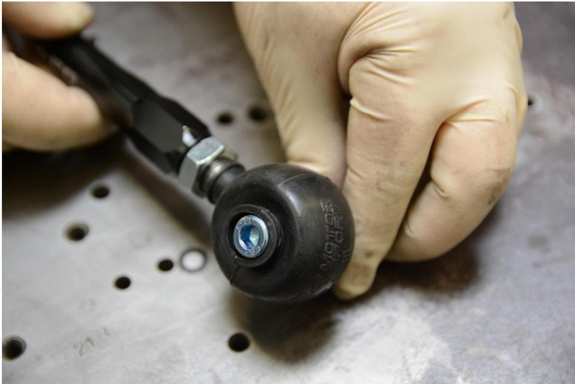
**Step 12** – Attach upper end of sway bar end link to the strut tab (as shown below) on the correct side of the tab. Do not put it on the incorrect side of the tab. Seriously, please install on the same side of the tab that the stock part was on. The hexagonal end of sway bar end link tube should be on the bottom, towards the sway bar.
