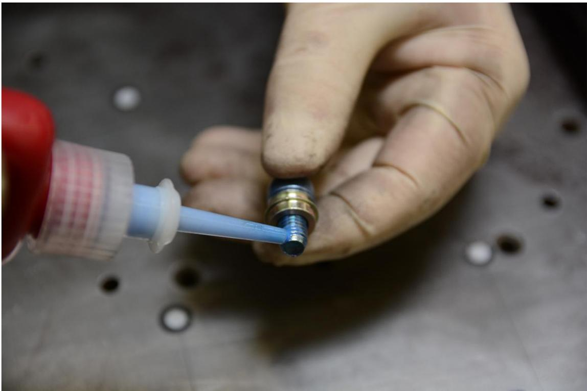
**Step 11** – Install Allen bolts and spacers into heim joints.
