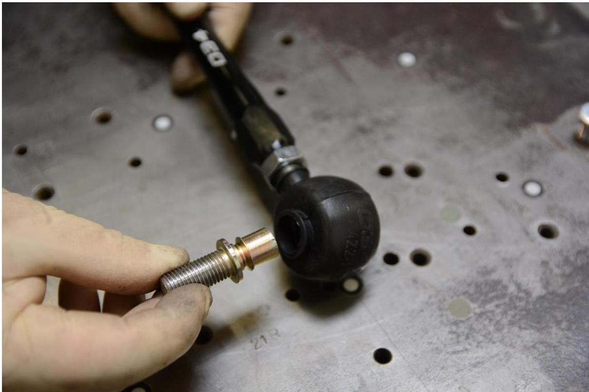
**Step 9** – Install spacer onto Allen bolt, taking note of the orientation shown below.
