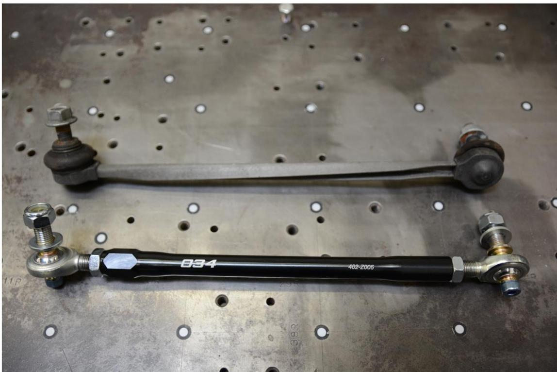
**Step 5** – (If using dust boots.) Disassemble the 034Motorsport End Links. Insert heim joint into dust boot. The boots will stretch to accommodate the heim, but avoid using sharp tools to pry at the boot.
