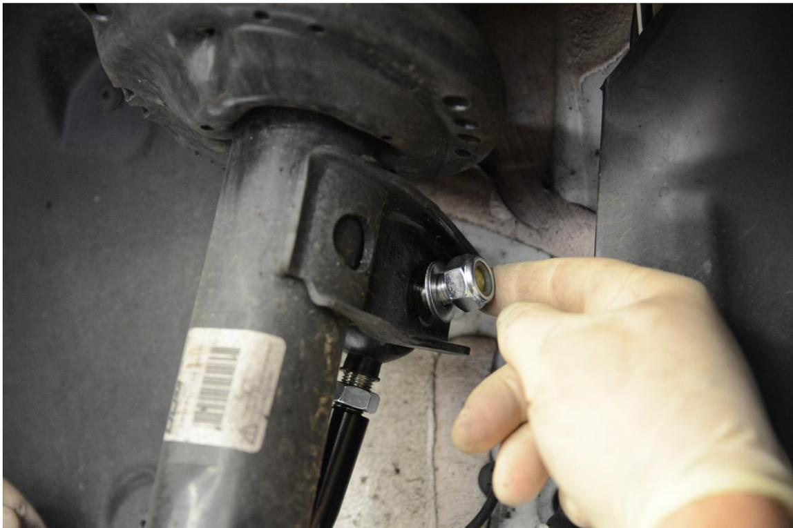
**Step 13** – Tighten nut and Allen bolt to 25 Nm using 6mm Allen Socket and 19mm Wrench.
