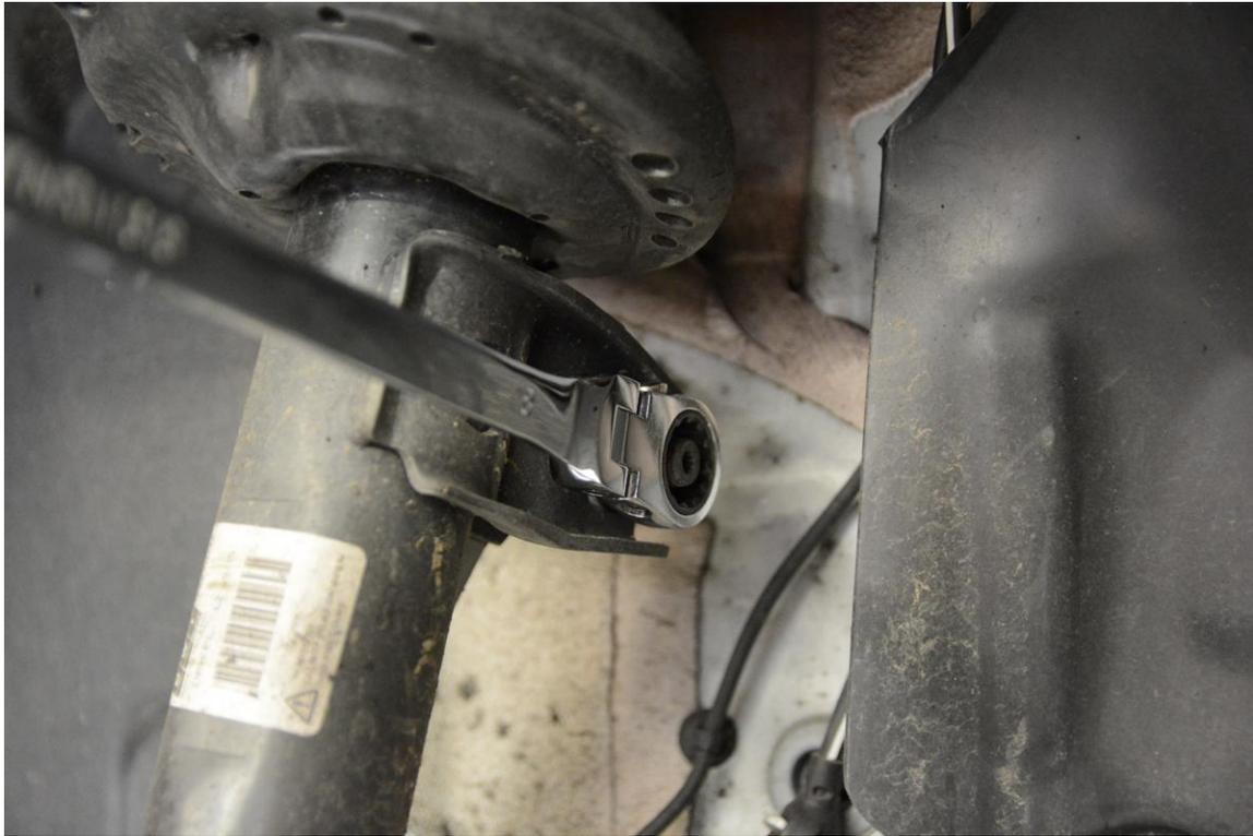
**Step 4** – (If you wish to use the supplied dust boots, please proceed to Step 5.) Set 034Motorsport End Link and Factory End Link side by side, and adjust the length of the 034Motorsport End Link to match. **Important:** Leave at least 8 threads exposed at the top portion (round tube, no hex) of the end link to allow for clearance at mounting tab.
