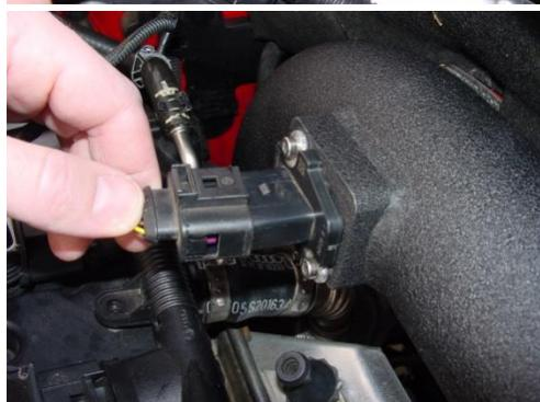
10. Install MAF sensor (fits one direction only) and tighten with two M4x8mm Philips head screws supplied. Attach electrical connector.
