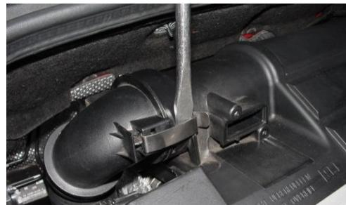
3. Unclip and disconnect turbo intake hose from air filter box.
