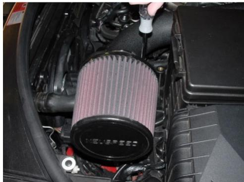
11. Install filter onto end of intake pipe.
