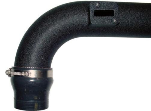
8. Install silicone hose onto turbo side of NEUSPEED intake pipe and tighten with #44 clamp supplied. NOTE: Screw clamp should be rotated toward passenger side of vehicle.
