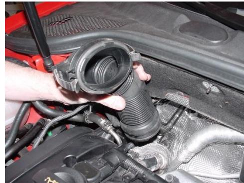
5. Remove turbo intake hose at turbo by squeezing spring clamp with spring clamp pliers. **CAUTION: Do not let any debris or objects fall into turbo inlet or damage may occur.**
