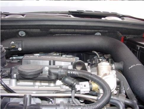
9. Install NEUSPEED intake pipe onto turbo inlet with #40 clamp supplied and attach rubber isolator mount to ear on end of cylinder head with M6x10mm screw. Intake pipe should be positioned at an upward angle toward brake fluid reservoir for engine torque clearance, now tighten hose clamp and M6 screw.
