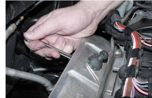
6. Installing NEUSPEED heat shield: First remove the (2) 10mm hex nuts located on bottom side of factory heat shield connecting the rear air filter box (engine cover) mounts. Then using a 24mm 12 point socket, unscrew the mounts.
