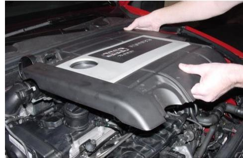
4. There are four rubber grommet mounts holding air filter box (engine cover) to engine. Lift up one corner of air filter box at a time to detach.
