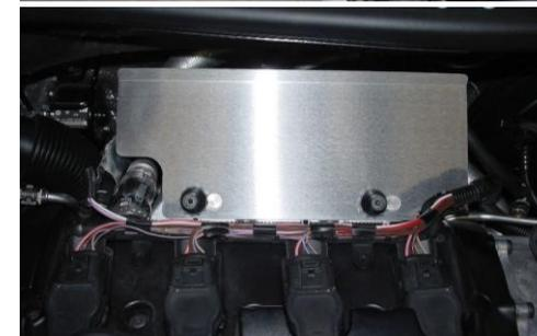
7. Install NEUSPEED heat shield using original air filter box mounts with SS washers supplied. Then reinstall 10mm hex nuts on bottom side.
