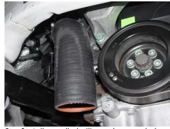
Install supplied silicone hose and clamp to turbocharger discharge adapter. Do not tighten clamp at this time.
