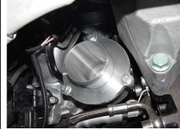
NEUSPEED billet discharge Install adapter using original bolts. Torque bolts to 4 - 5 ft. lbs.
