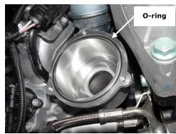
Make sure O-ring is properly seated in groove of turbocharger housing. Use grease to retain in groove if necessary.
