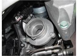
Unbolt original discharge adapter and separate adapter from turbocharger, (3) 10mm hex bolts. Note: Use caution not to damage O-ring.
