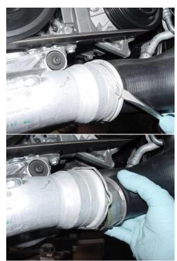
Use screwdriver to pull-out clip to release rubber intercooler hose from aluminum pipe.
