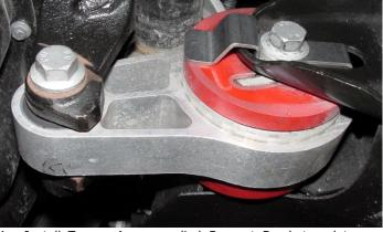
Install Torque Arm, supplied Support Bracket and torque 4. bolts to 80 foot/pounds (108nm). Double check installation.
