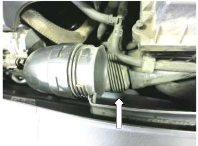
f. Disconnect the air duct from the lower air box and remove from vehicle. **Note: Removing the duct allows for easier air box removal.**
