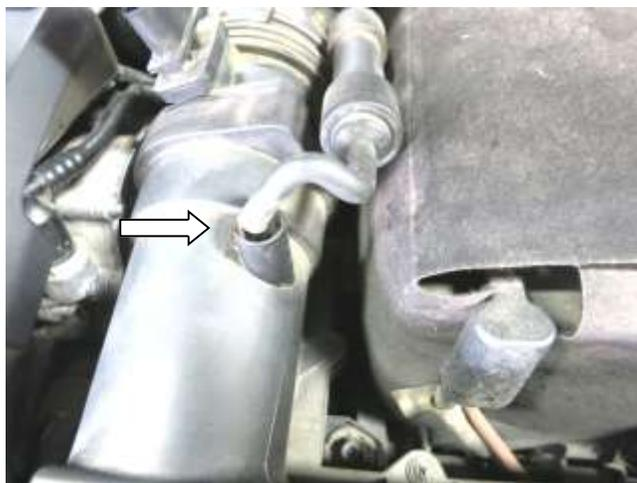
b. Disconnect the vacuum line from the factory air inlet tube.
