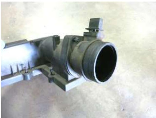
c. Remove the MAF sensor from the factory air box. The MAF sensor is secured with 2 Philips screws.
