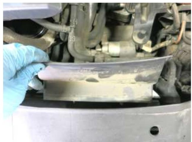
h. Remove the two screws securing the fresh air inlet to the core support and remove it from the vehicle.
