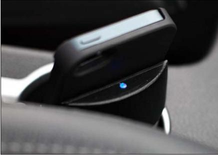
When Inserting a Qi compatible smartphone charging begins automatically and the LED turns from red to blue
