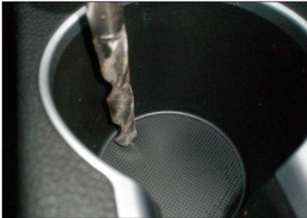
=> If the cup holder has a solid bottom you have to drill a hole (diameter of 18 mm) in order to install the USB connector cable
