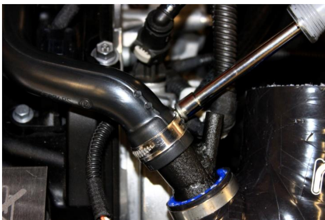
16. Connect breather hose with 25mm clamp supplied.
