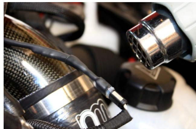
22. Heat shrink on supplied tubing to both connectors to weather seal.
