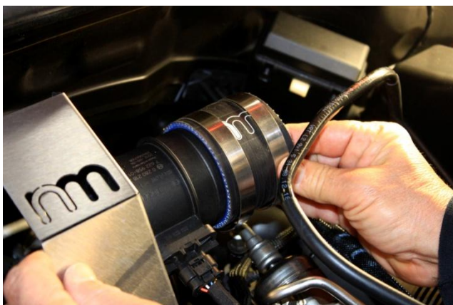
18. Install and tighten silicone hose coupler onto MAF sensor using supplied #44 hose clamp.
