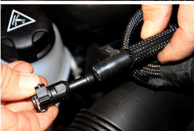
6. Disconnect any wire harness and hose supports on intake tube then loosen clamp at turbo and remove.
