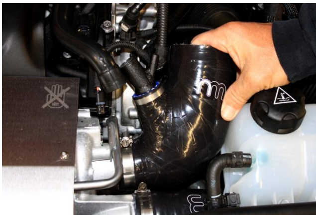
15. Loosely install silicone turbo inlet hose onto turbo using supplied #28 hose clamp. NOTE: Do not tighten at this time.
