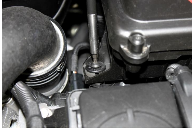
4. Remove T25 TORX screw located on passenger side of air filter box and lift off. NOTE: There are [3] pin mounts that are pushed into rubber grommet mounts on intake manifold, so effort may be required to lift air filter box off of mounts.
