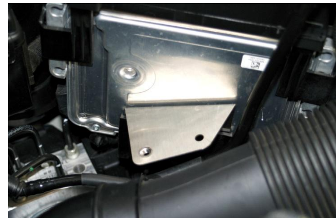
11. 2011-3/2012 EARLY N18 Remove protective film from double-sided tape on stainless steel fresh air hose bracket. Slide bracket down between ECU and black plastic ECU mount, while keeping double stick tape from touching. With bracket pushed all the way down, press against ECU.
