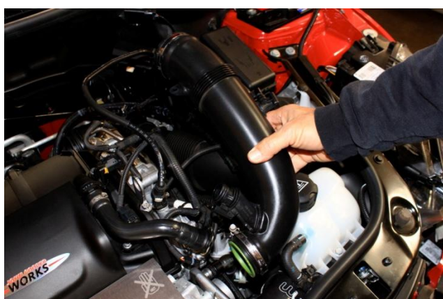
6. Disconnect any wire harness and hose supports on intake tube then loosen clamp at turbo and remove.
