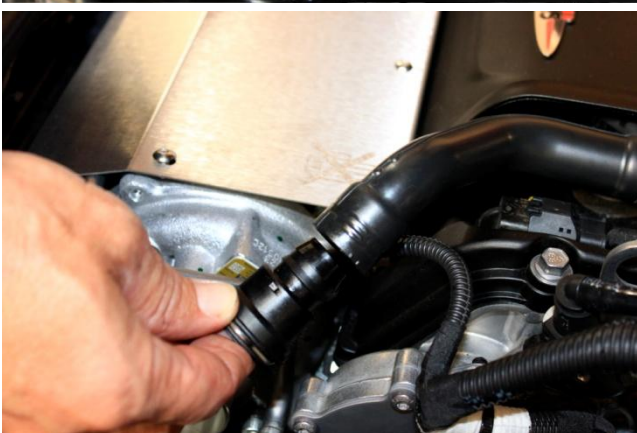
4. Remove T25 TORX screw located on passenger side of air filter box and lift off. NOTE: There are [3] pin mounts that are pushed into rubber grommet mounts on intake manifold, so effort may be required to lift air filter box off of mounts.
