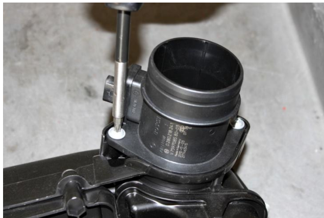
6. Disconnect any wire harness and hose supports on intake tube then loosen clamp at turbo and remove.
