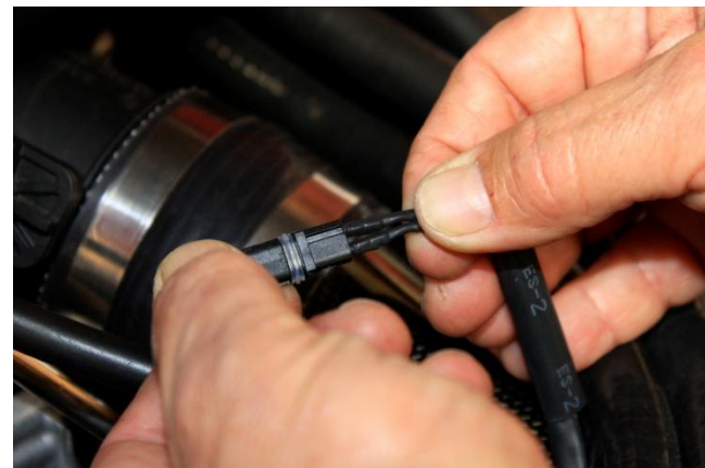
21. Locate previously disconnected heater wires from breather hose and vent hose. The supplied resistor harness connects to the front connector that attached to the valve cover breather hose. The other supplied resistor harness connects to the rear connector that attached to the vent hose on the factory intake pipe.
