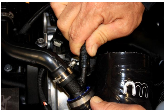
17. Install vent hose to "Y" breather adapter. NOTE: Spray inside of hose with WD-40 or equivalent to ease installation.
