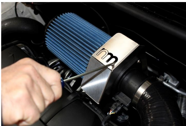
20. Using degreaser or contact cleaner and shop rag, clean inner mounting flange of NM filter. Install NM filter onto MAF sensor and tighten with long skinny screwdriver thru logo cut-out or from back side of bracket.
