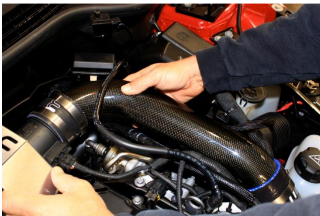
19. Loosely install supplied #44 clamps onto both silicone hose ends, then install air intake pipe into silicone turbo inlet hose first and then into MAF sensor hose. Adjust as necessary for clearance, paying close attention to clearance of silicone turbo inlet hose and coolant reservoir bottle. Tighten all clamps. NOTE: Do not forget to tighten #28 hose clamp from Step 14. Connect breather hose to cylinder head cover.
