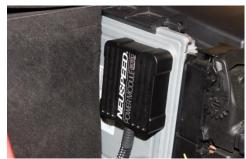
Clean surface on side of ECU just in front of battery and stick-on NEUSPEED Power Module with supplied Velcro. Route wire harness toward engine underneath air intake hose between air filter box and turbo.
