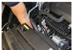
A3/GTI/GOLF: Boost sensor is a little harder to access. Either reach down in front of alternator to just below A/C compressor to get to boost sensor in Air Charge Pipe or see step#8.
