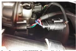
Connect NEUSPEED Power Module harness in-line as shown.
