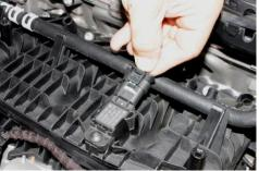
Squeeze locking tab on end of MAP connector then disconnect electrical connection. TIP: Push in on connector while squeezing tab. Repeat for Boost sensor.
