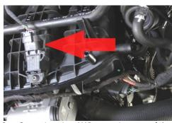
Sensor Location: MAP sensor is on top of the intake manifold (shown). Boost sensor is on the plastic Air Charge Pipe located just below the A/C compressor.
