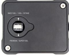
11. NEUSPEED Power Module has a (2) position power switch access from the back side. DOWN position for Premium fuel 91+ octane (5PSI increase) and UP position for 100+ Race fuel (7PSI increase). NOTE: Only use RACE setting when fuel in gas tank is 100 octane or higher.
