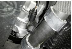
S3/GOLF R: From underneath vehicle remove lower engine splash pan (T25/T40 Torx Screws) to access boost sensor in Air Charge Pipe just below A/C compressor.
