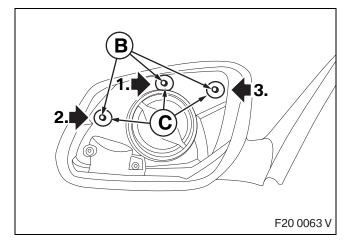
Note the sequence when screwing the components into place. ◀
