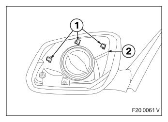
Break off the three lugs (1) from the mirror casing (2).
