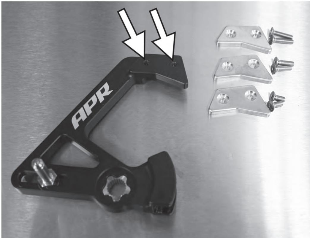
15) Select the amount of inertia weight you wish to use. Select the appropriate length screws for the number of weights used. When installed, the screws should not protrude from the bottom of the primary lever. Install the weights to the primary lever, and tighten the 4mm allen screws to 2Nm (18in-lb).
