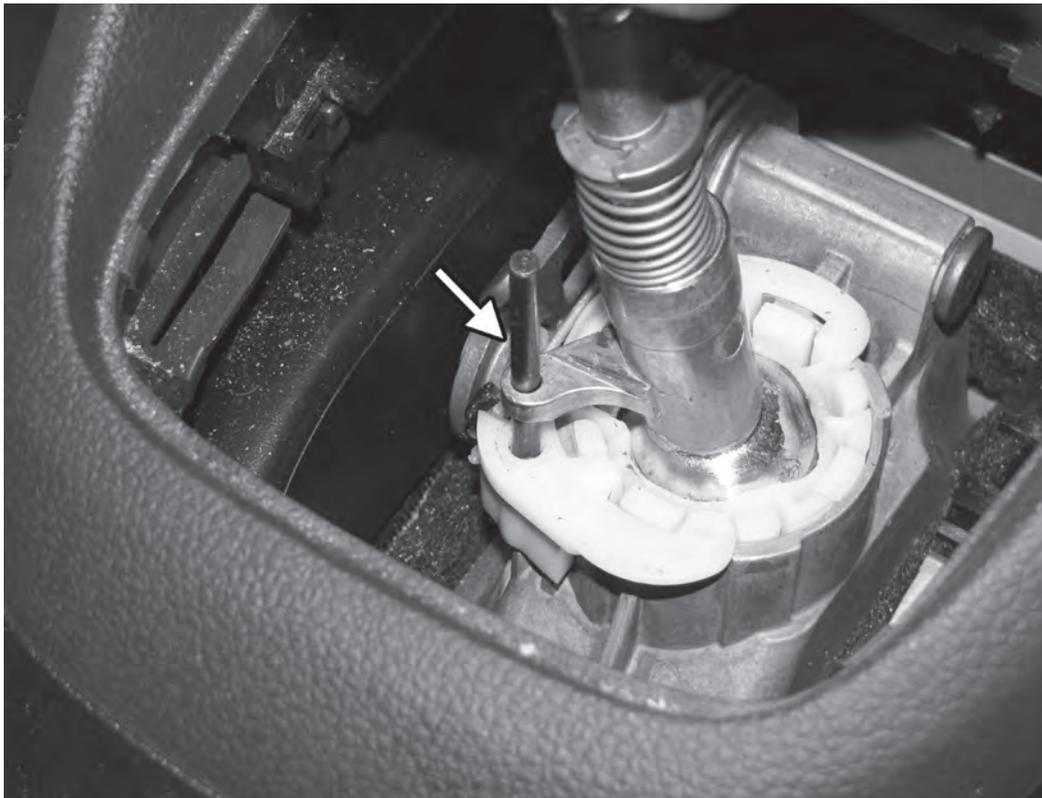
31) Remove the locking pin from the shifter inside the car. Replace the sound deadening absorber and reinstall the shifter surround trim by pushing the securing clips back in place. Make sure the shifter freely goes into each gear, including reverse.
