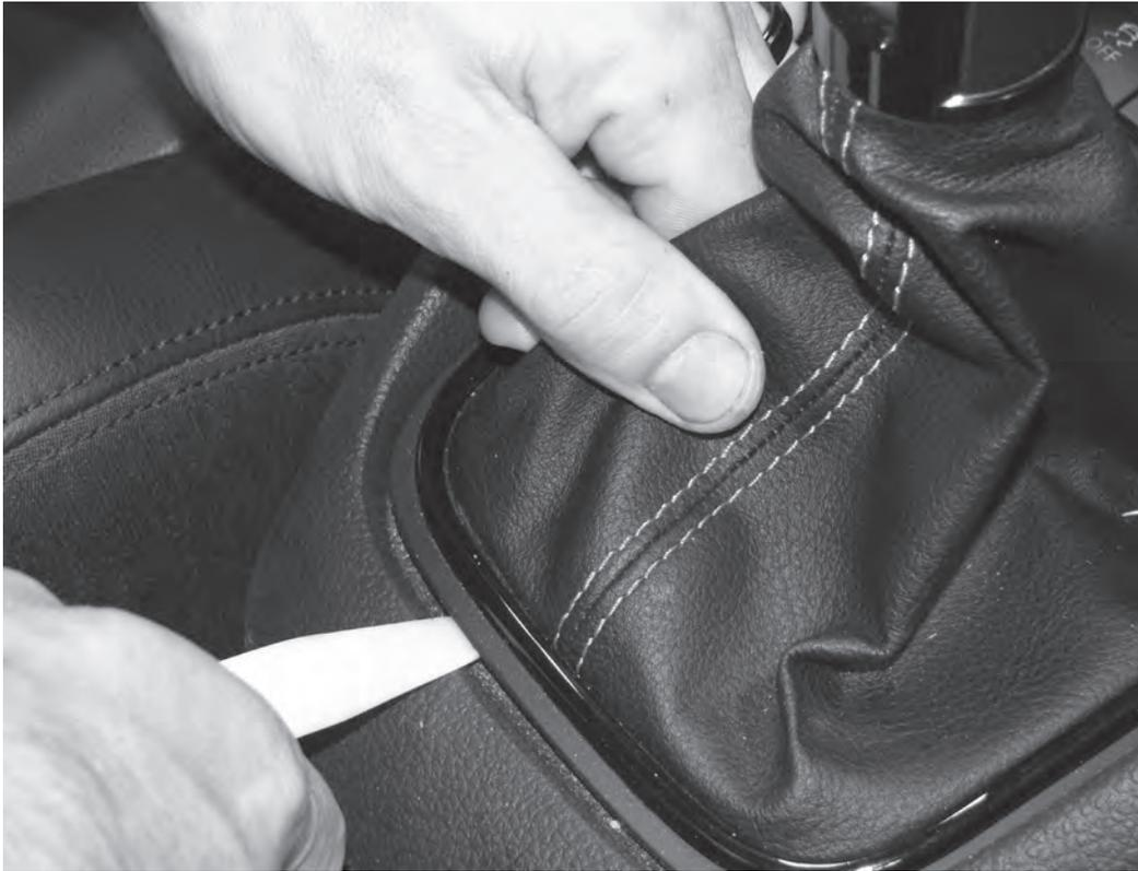
21) Inside the car, gently lift up on the boot around the shifter, and then using a plastic trim tool, carefully pry the shifter surround trim up. There are two locking tabs on the back of the shifter trim.
