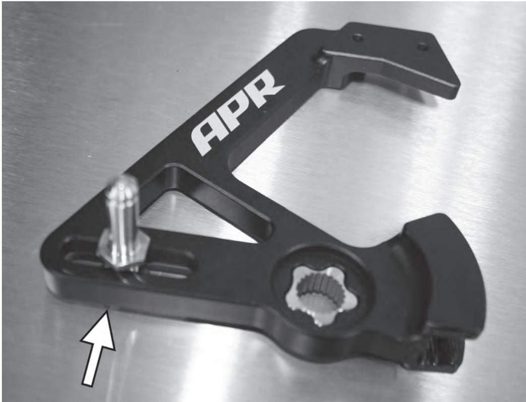
13) Select and install the appropriate cable post onto the primary lever, and loosely secure with a 13mm locknut.
