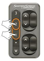
Now select which speed you want to adjust by pressing the Speed #2 " 2" Button, or the Speed #1 " 1" Button.
