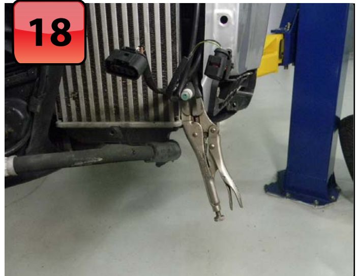
Pinch the washer fluid lines with soft-jawed pliers or a hose clamp. Slide two lengths of scrap rubber hose over the jaws of your needle-nosed vise grips to make a good hose clamp.
