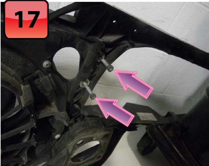
The crash sensors bolt to the radiator support with two Allen head screws. Our photo shows the bolt locations on the right side with the sensor already removed.
