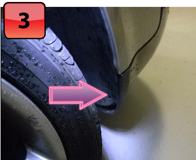
To access and remove the nuts from the three threaded studs on each side of the bumper fascia, (where it joins the bumper), remove the lower retaining screw from each fender liner (arrow). Pull the liner back to expose the nuts, and remove them with a 10 mm socket.
