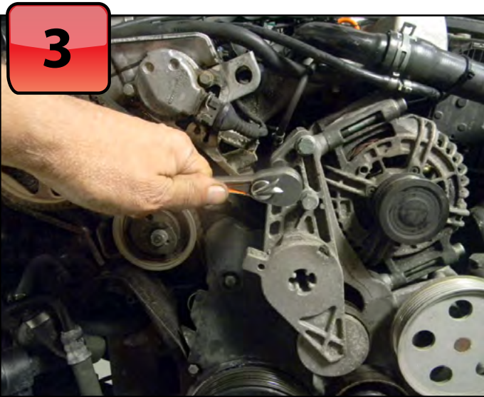
With the accessory belt removed, unbolt the tensioner assembly and remove it. Three bolts.
