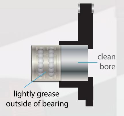
press in bearing with 78mm Plate
