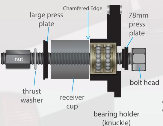
Assemble the tool as shown. Lube threads, nut, and washer with grease.
