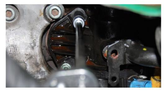
As the second 10mm bolt is removed, the thermostat will separate from the engine block, allowing coolant to flow out from underneathe it.
