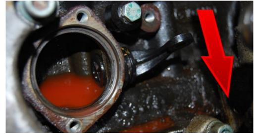
To help remove the j-plug from the thermostat housing inlet body, use a ratchet extension or similar tool to push on the j-plug from inside the inlet while gently twisting the plug outwards. The factory j-plug o-ring may be swollen making the plug difficult to remove. Use caution and patience to slowly unseat the j-plug from the engine block, while pressing on it from inside the thermostat inlet body.
