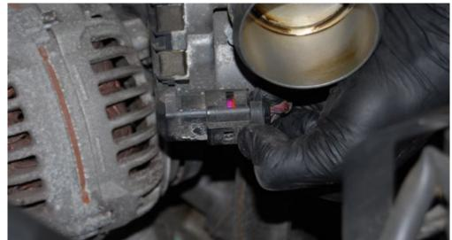
Remove the four 5mm Hex bolts that secure the throttle body to the intake manifold using a ratchet with short extension.
