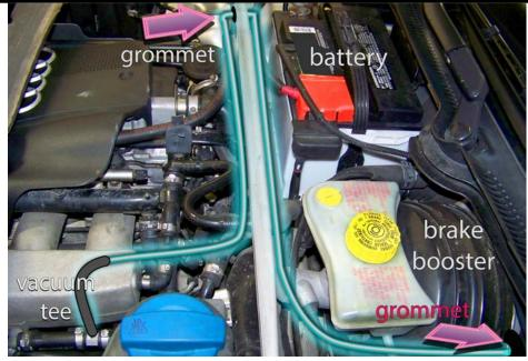
Use the zip ties in the kit to secure the plastic line at several locations. Leave a slight bend in the rubber braided hose at the vacuum tee to compensate for engine movement and vibration.
