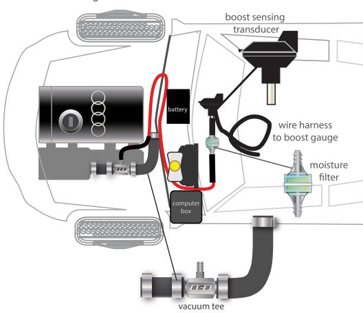
The vacuum tee, plastic line, clamps, and braided rubber hose are all included in your kit. Use the zip ties to secure all lines and hoses safely away from moving components, like pedals and the steering mechanism.
