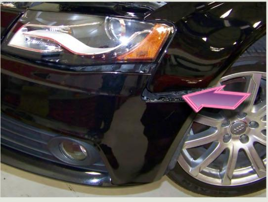
Lower the car and align the top of the bumper with the headlights. Close the hood to check the grille face-to-hood alignment.
