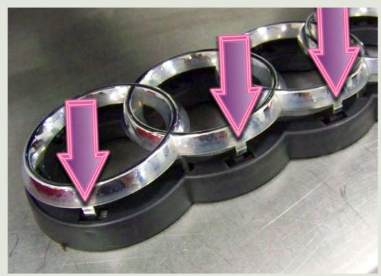
Attach the Audi emblem support to the grille. Use the straps and screws in the kit. Lay the straps across the back of the grille. Insert the screws through the slots in the straps and mesh openings; then screw them into the raised screw posts on the back of the emblem holder. Alternately tighten the screws to pull the straps tight against the grille mesh; just don't overtighten.
