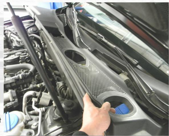
Carefully remove the cowl panel by releasing the center retainer, lifting up at both sides and pulling it towards the front of the car.
