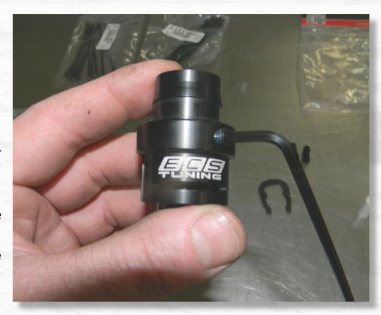
Apply loctite onto the nipple threads.
