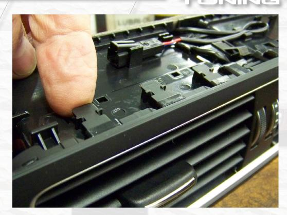
Pop off the center trim panel at the vent control rollers. This is a snap-inplace piece, so work carefully to avoid damaging it.
