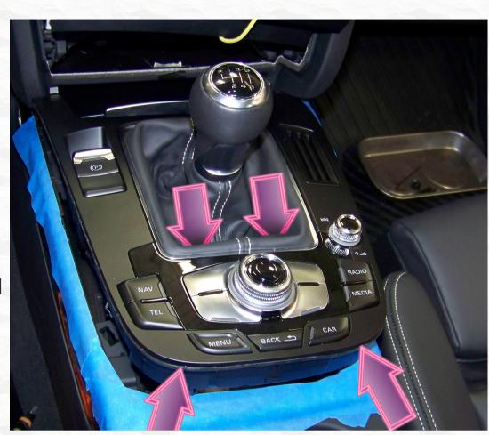
Remove the two screws holding the ashtray assembly in the console (locations indicated by arrows). Then slide the ash tray assembly toward the shifter, out of the console.
