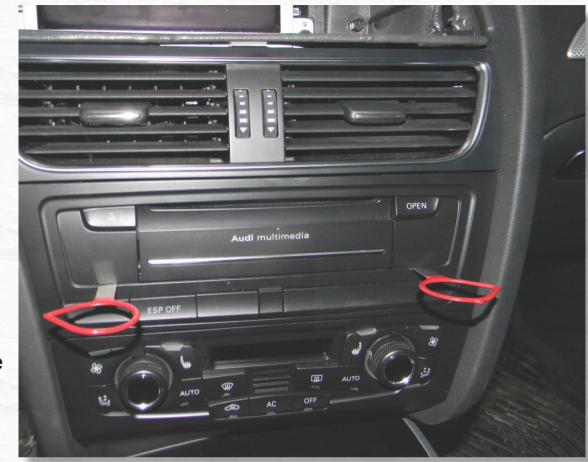
Using the Radio removal tools, slide the radio out so the center vent can be removed.
