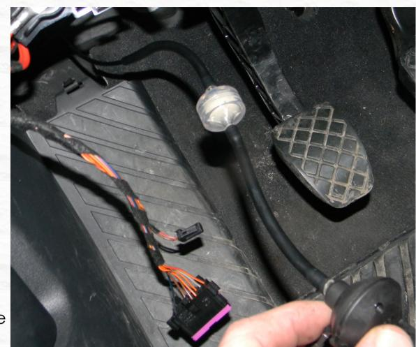
Trim the rigid plastic tubing and install the vacuum transducer as shown using two pieces of the flexible vacuum hose and the inline filter.
