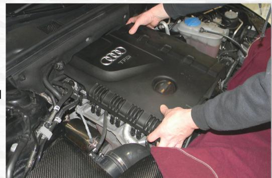
Disconnect the PCV hose at the intake manifold by squeezing the retainer tabs together and pulling the hose off of the intake manifold.
