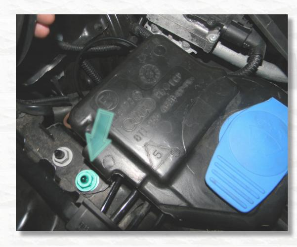
Remove the ECU cover by removing the three Torx T30 screws and lifting the cover off.
