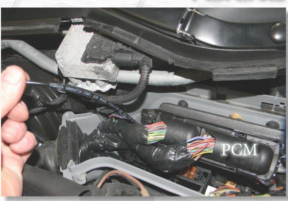
Locate the rubber wiring boot for the ECU harness.
