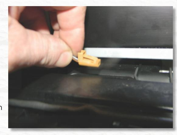
Unplug the electrical connector from the top of the center outlet vents.
