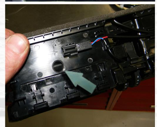
Drill a 12mm hole in the main vent housing at the location shown in the photo.
