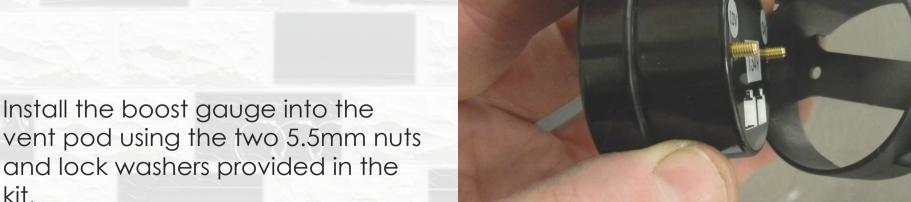
vent pod using the two 5.5mm nuts and lock washers provided in the kit.
