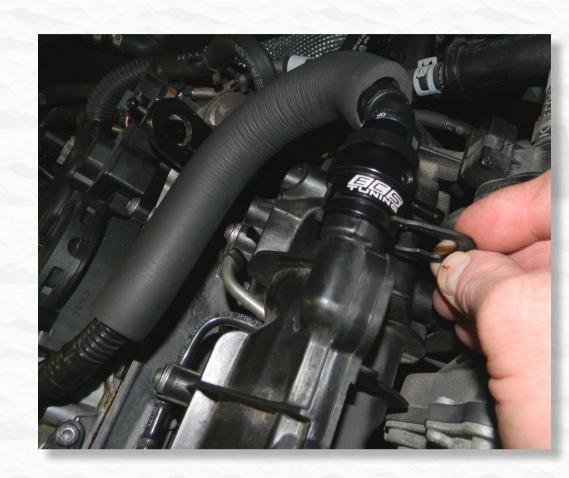
Note the position of the Boost Tap. The nipple should angle slightly downward, as shown in the picture.
