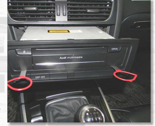
Note: The radio does not need to be completely removed, but be careful not to slide it out too far so it falls onto the console.
