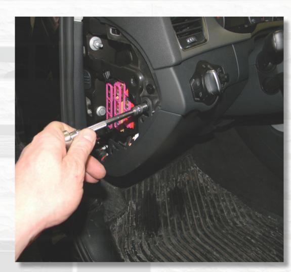
Remove the 8mm bolt on the LH side of the driver's lower dash panel.
