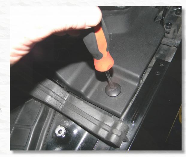
Remove the plastic retainers from each side of the cowl panel using a flat blade screwdriver.
