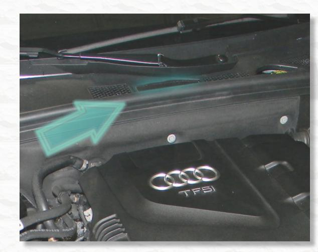
Moving back to the engine bay, remove the battery positive connection access panel in the center of the cowl.
