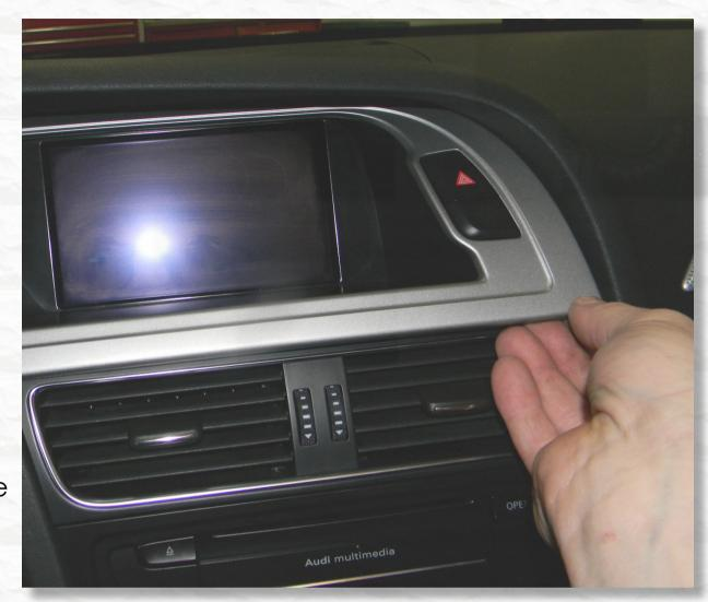
Remove the upper RH dash trim piece by pulling out on the bottom of the trim piece to release the clips.
