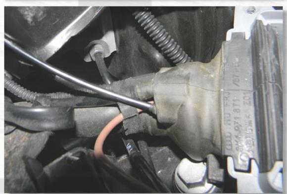
Route the tube through the foam seal just in front of the ECU housing.
