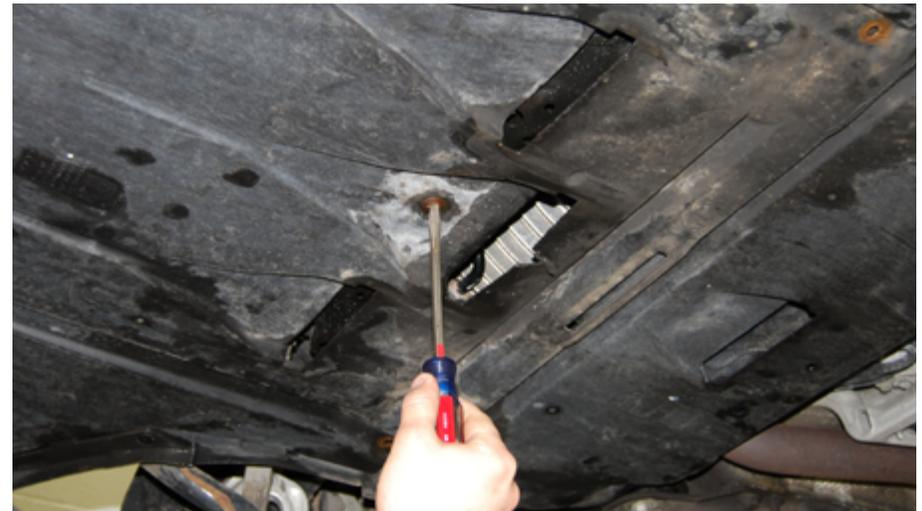
Remove the passenger side belly pan screw.
