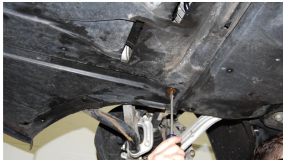
Remove the driver side belly pan screw.
