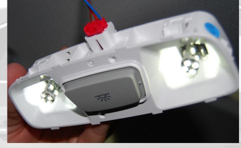
Clip the two halves of the rear dome assembly together, and reinstall the bulb assembly into the vehicle.
