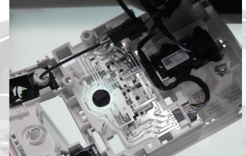
Remove the incadecent bulb and replace with a T10 Base Cool White 8 Chip LED Bulb. Slide the LED in place and press the dome light 'on' button to check that the polarity is accurate.
