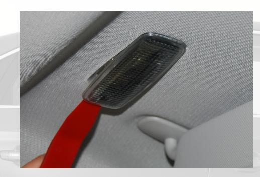
Do not pull with excessive force on the unit; if you are prying at the correct side, the assembly will fall out with little effort.
