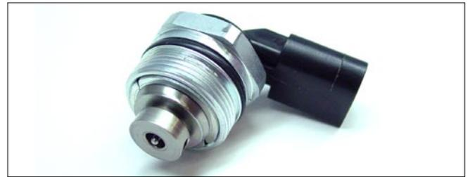
5. Carefully remove the valve, and the metal disk below it in the fuel pump housing. Save these for later re-assembly on your clean workspace. Be careful with the small disk it is actually 3 pieces.
