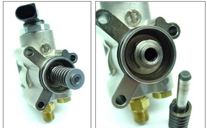
2. Place the return spring and piston on your clean workspace. Once these items are removed from the pump, a Stainless nut will be revealed. Use your 18mm. socket to loosen and remove the Stainless nut (it's actually the seal holder too!), and place it on your clean workspace.
