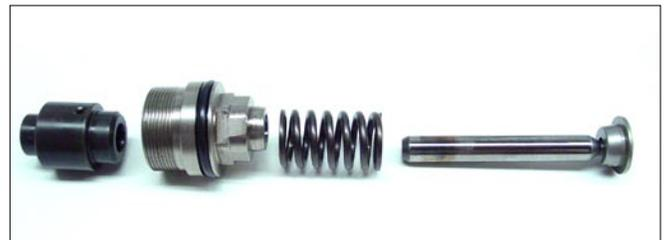
3. Inside the Seal Holder, is the OEM cylinder that can be put aside, along with the OEM piston. The only part you will be re-using from the mechanical side of your High Pressure Rail Pump is the Stainless Seal Holder.
