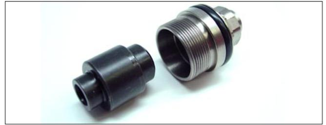
4. Continue to dis-assemble your pump by removing the pressure relief valve with your 32mm. Open end Box Wrench.
