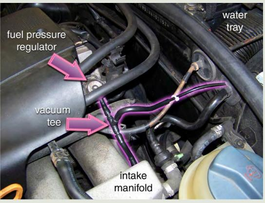
Vent Pod Boost Gauge Installation
