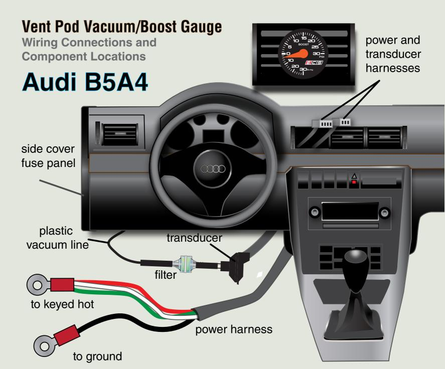
Vent Pod Boost Gauge Installation
