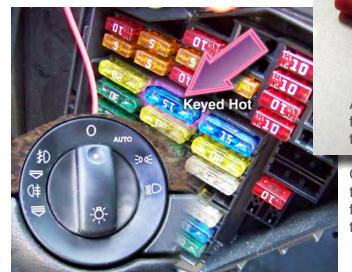
Attach the fuse tap to the fuse as shown and reinsert the fuse.
