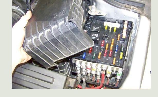
Using a 10mm socket, remove the nut on the fuse block stud that is fourth from the right.
