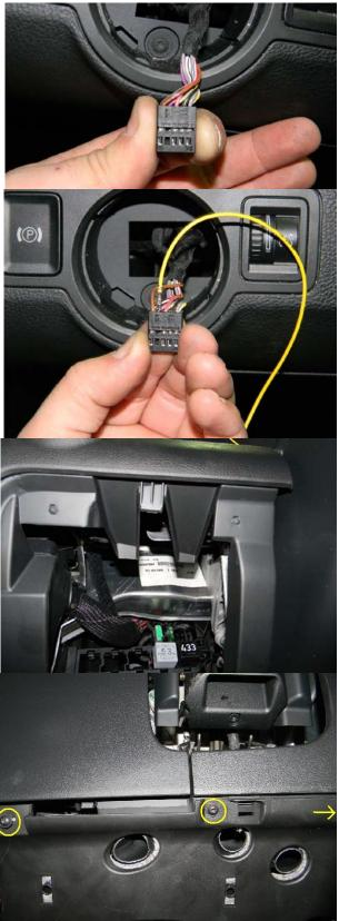
14. Take off the OBD2 connector and remove the light so the plastic cover can be removed from the car for easier access to under the dash.
