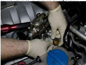
**8.** Install the two (Large and Small) 90\* port adapters, and secure to oil separator and valve cover with quick release clamps.
