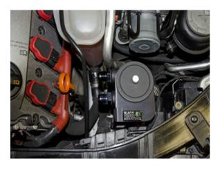
**7.** Attach the two sets of adapter rings (4 pieces – Two halves of each) and attach them to both the port on the valve cover and the oil separator.
