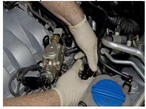
**9.** Install the two supplied hoses to the port adapters and the catch can fittings. Tighten each using the adjustable wrench.
