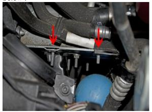
5. Mount the bracket behind the drivers side headlight, along the frame rail as pictured. Bolt the bracket to the frame rail using the existing 6mm (10mm socket) nut as well as the supplied 6mm nut and washer.
