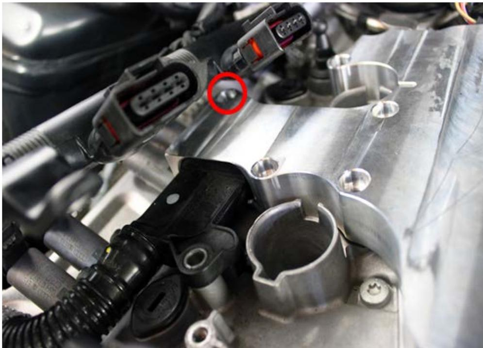
**Step 8** – Secure the Valve Cover Breather Adapter to the valve cover using the supplied M6x25 Bolts. The M6X22 Bolt goes into the left-most hole circled above. Secure the PCV assembly to compressor inlet tube to the valve cover using the factory T27 Torx screw.
