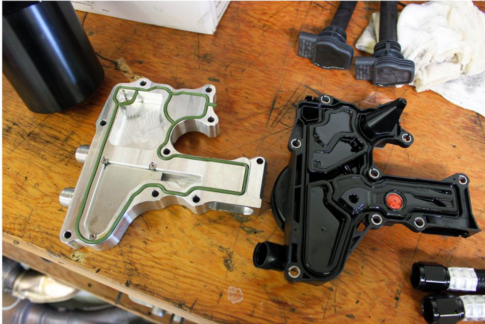
**Step 7** – Position the 034Motorsport Valve Cover Breather Adapter such that the holes align with the threaded holes in the valve cover, and push the PCV assembly to compressor inlet tube into it until it seats.
