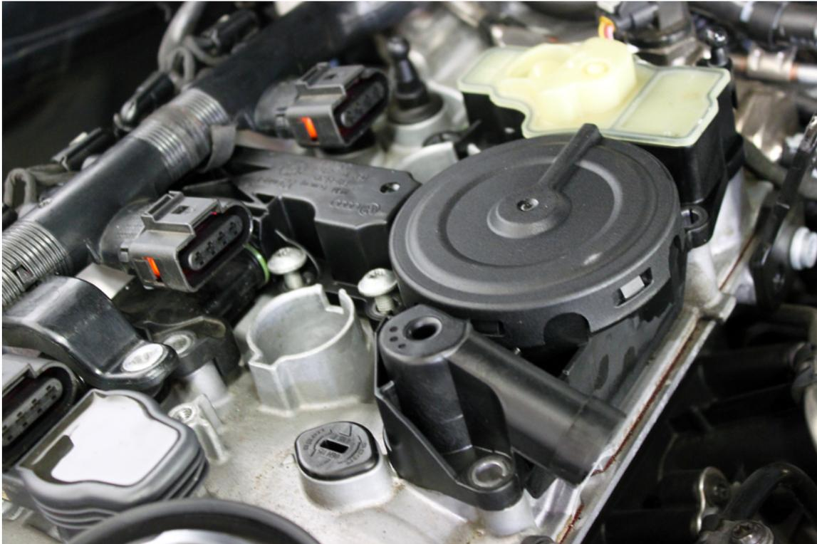
**Step 6** – Remove the factory rubber seal from the PCV assembly, and install it into the Valve Cover Breather Adapter.
