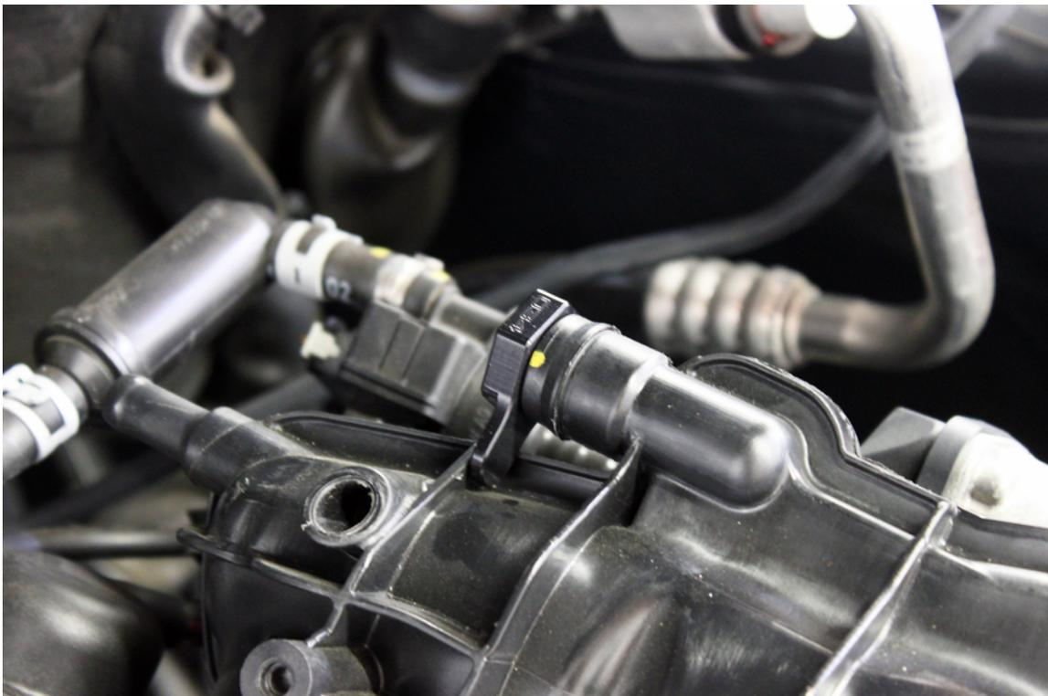
**Step 4** – Unbolt the T30 Torx screw securing the coil harness loom, and unplug the coil harness from all 4 coils. You can now access the single T25 Torx screw securing the PCV assembly to compressor inlet tube to the valve cover. Remove the T25 Torx screw and pull to remove the tube from the PCV assembly.
