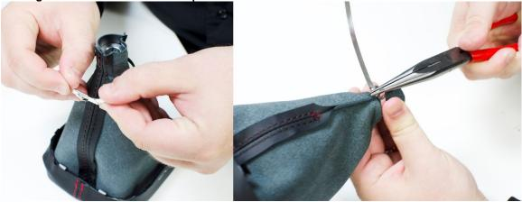
10. Using a sharp blade (x-acto knife) trim away any ecess flashing from the boot once the clamp is tightened, you just need to trim away enough to allow access to the set-screw holes.
