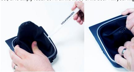
2. With the boot and inner trim ring removed, flip the boot to its underside, and loosen and remove the
