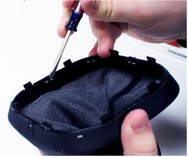
3. Once the Staples are removed, pull the boot apart from the ring (it should just fall apart).
