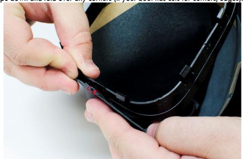
7. Using a heavy duty stapler (a regular stapler will not be sufficient for Manual shift rings, but would be fine for most DSG/Auto Rings), Periodically staple the boot to the trim ring like the factory boot. This step is optional as the adhesive is strong enough to hold the boot in place without staples.
