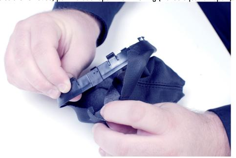
4. Using the supplied double-sided adhesive, place strips around the inside of the BFI boot, using smaller multiple pieces instead of larger continuous pieces. Be sure to reserve some of the tape to fill in gaps and folds where necessary.
