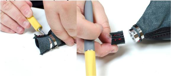
11. Simply invert the boot back to normal and you can insert the boot and trim ring back into the car
