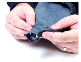
9. Using the supplied metal zip tie, clamp the boot to the shift knob adapter. Use the pliers to tighten the zip tie, twisting the end as shown to clamp it down. Cut off the excess.
