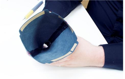
6. Peel the tape backing away as you start to attach the new BFI boot to your trim ring, peeling the tape as you work your way round the trim ring. Please note that the trim ring has designated spots for the seams to be placed, locate those indentions and put the seams there. Once in place use any extra adhesive to tape down and fold over any corners (if your boot has cuts for corners/edges).
