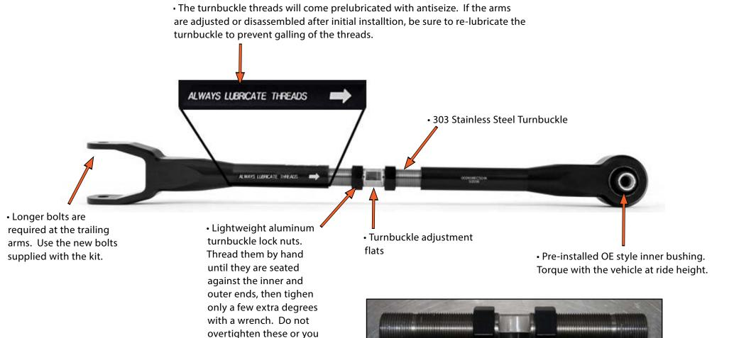
The turnbuckle should be evenly spaced between each half of the control arm. When adjusting, do not extend the control arm halves beyond the grooves (arrows) cut in the turnbuckle threads.
